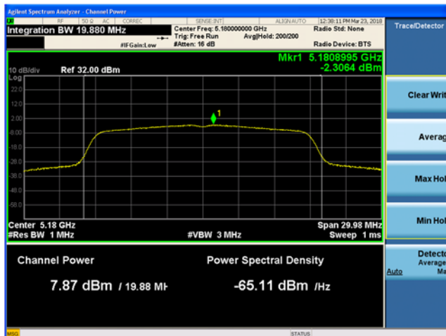
Plot 9-106. Maximum Conducted Output Power and PSD, Diversity Antenna 802.11n HT20 (Ch. 36)
