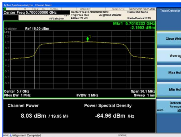
Plot 9-84. Maximum Conducted Output Power and PSD, Main antenna 802.11n HT20 (Ch. 140)
