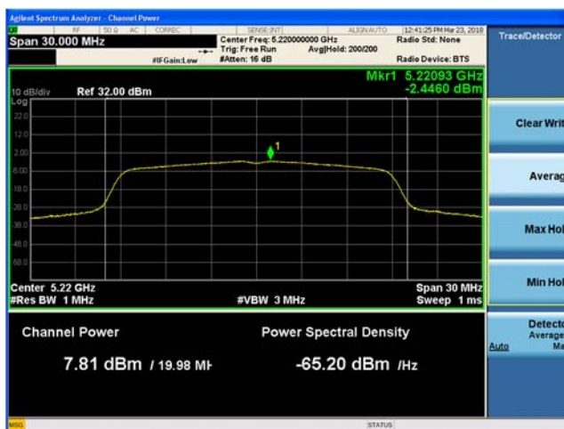
Plot 9-107. Maximum Conducted Output Power and PSD, Diversity Antenna 802.11a HT20 (Ch. 44)
