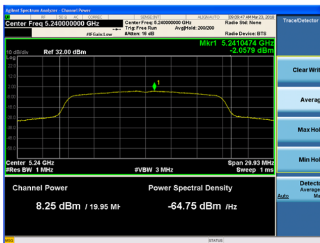
Plot 9-78. Maximum Conducted Output Power and PSD, Main antenna 802.11n HT20 (Ch. 48)
