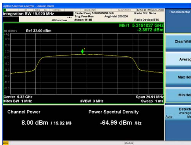
Plot 9-111. Max Conducted Output Power and PSD, Diversity Antenna 802.11n HT20 (Ch. 64)
