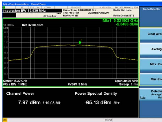
Plot 9-81. Maximum Conducted Output Power and PSD, Main antenna 802.11n HT20 (Ch. 64)
