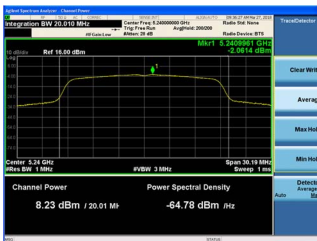
Plot 9-108. Maximum Conducted Output Power and PSD, Diversity Antenna 802.11n HT20 (Ch. 48)
