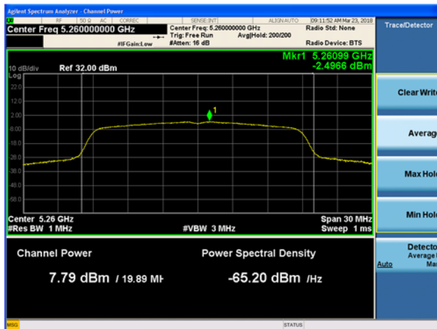
Plot 9-79. Maximum Conducted Output Power and PSD, Main antenna 802.11n HT20 (Ch. 52)
