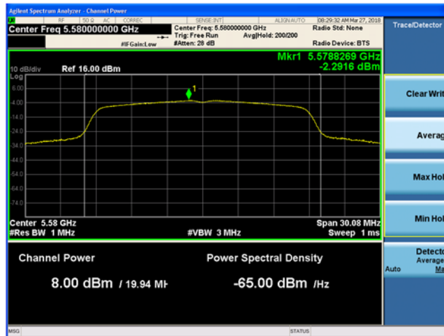
Plot 9-83. Maximum Conducted Output Power and PSD, Main antenna 802.11n HT20 (Ch. 116)
