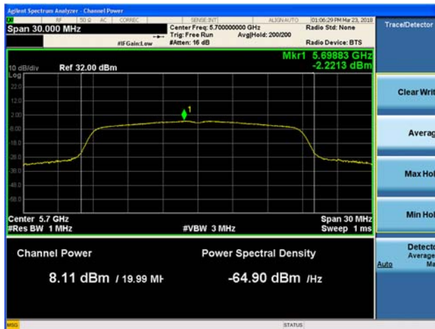
Plot 9-114. Max Conducted Output Power and PSD, Diversity Antenna 802.11n HT20 (Ch. 140)
