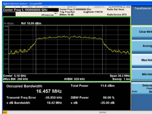
Plot 9-1. 26-dB Emission Bandwidth and 99% OBW, Main Antenna 802.11a (Ch. 36)
