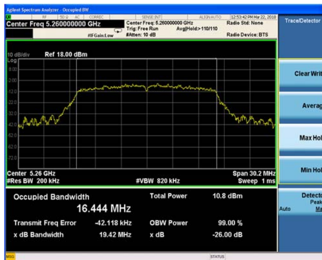
Plot 9-4. 26-dB Emission Bandwidth and 99% OBW, Main Antenna 802.11a (Ch. 52)
