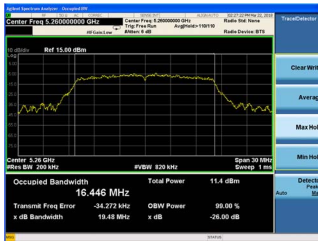
Plot 9-28. 26-dB Emission Bandwidth and 99% OBW, Diversity Antenna 802.11n HT20 (Ch. 52)
