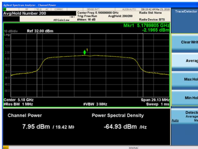
Plot 9-61. Maximum Conducted Output Power and PSD, Main antenna 802.11a (Ch. 36)
