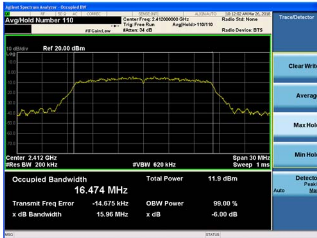
Figure 9-9 99% Bandwidth 802.11g - Ch.1 (2412 MHz)
