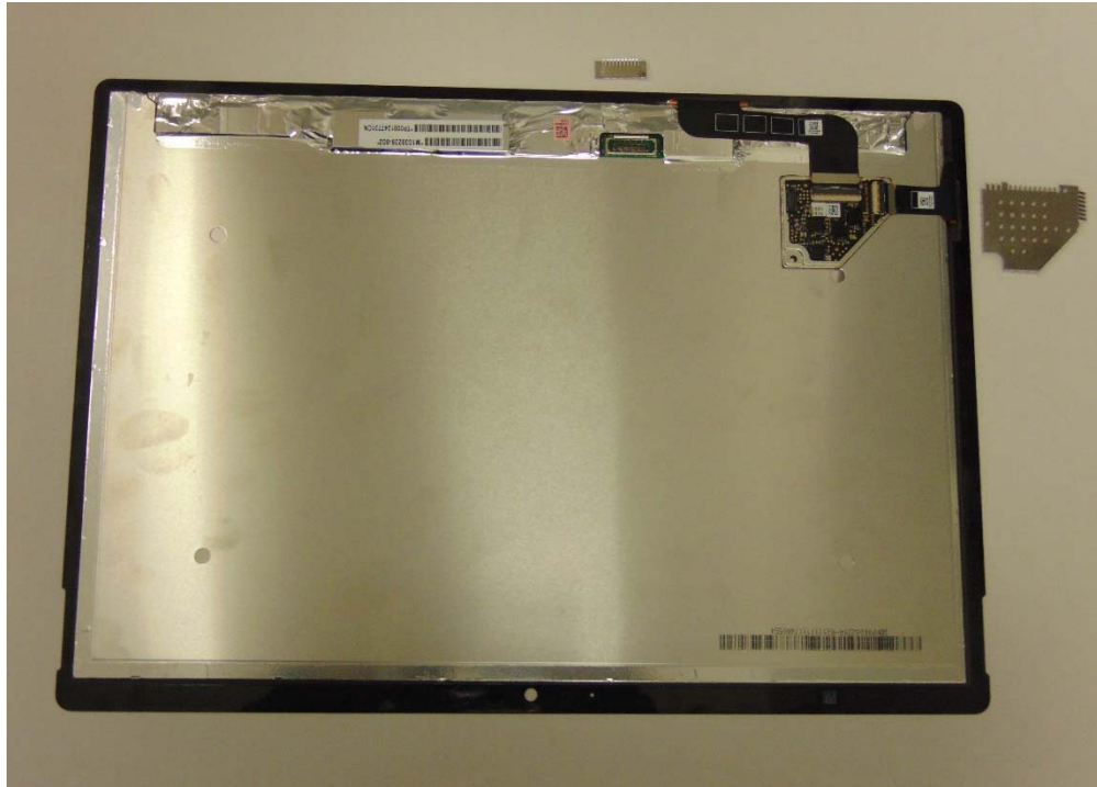
Display with shield cans removed
