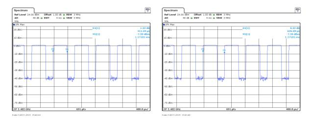
T<sub>on</sub> =411.59 μs T=626.09 μs
