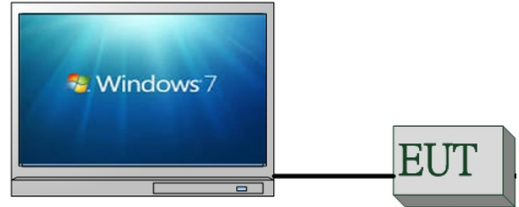
Fig.2-3 Conducted Emission (Antenna Port) Configuration
