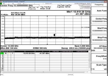
18G-23GHz Spurious Emission Test Data CH-Mid
