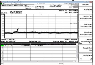
18G-23GHz Spurious Emission Test Data CH-High
