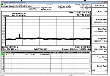
8G-13GHz Spurious Emission Test Data CH-High
