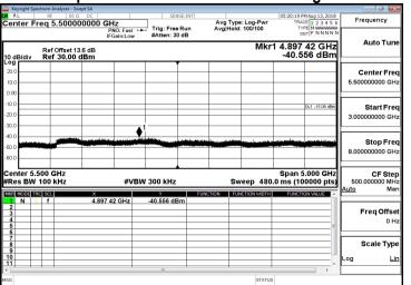
18G-23GHz Spurious Emission Test Data CH-High
