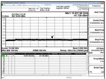
18G-23GHz Spurious Emission Test Data CH-High
