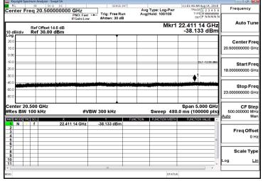
23G-26.5GHz Spurious Emission Test Data CH-Mid
