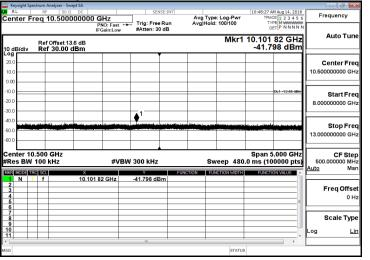
13G-18GHz Spurious Emission Test Data CH-Mid
