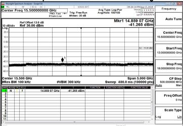
3G-8GHz Spurious Emission Test Data CH-High
