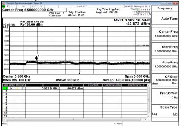
8G-13GHz Spurious Emission Test Data CH-Mid
