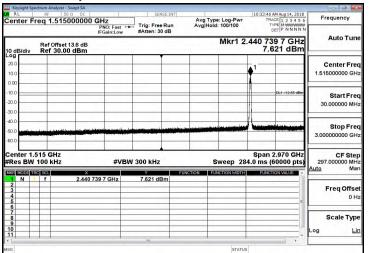
3G-8GHz Spurious Emission Test Data CH-Mid
