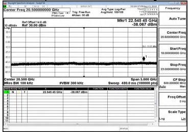
8G-13GHz Spurious Emission Test Data CH-High
