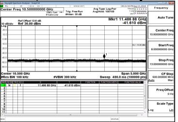
23G-26.5GHz Spurious Emission Test Data CH-High
