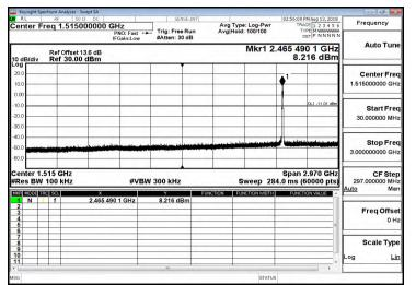
13G-18GHz Spurious Emission Test Data CH-High
