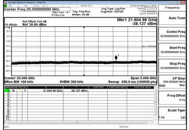
23G-26.5GHz Spurious Emission Test Data CH-High
