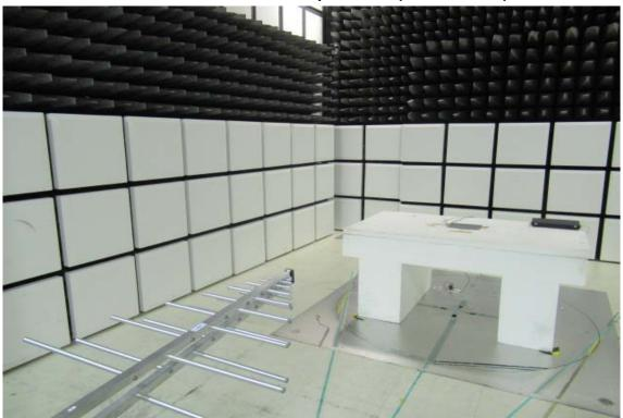
Radiated Emission Set up Photos (Below 1GHz)
