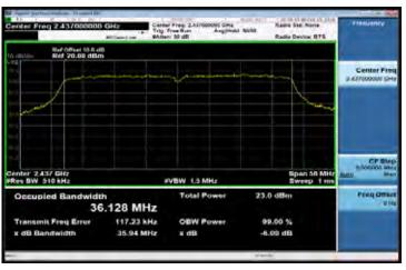
99% Band Width Test Data CH-High 2462MHz
