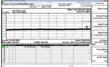
8G-13GHz Spurious Emission Test Data CH-Mid
