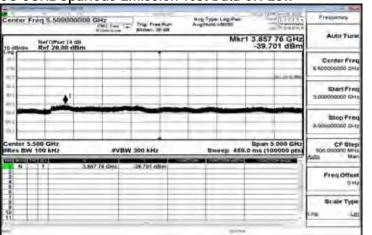
18G-23GHz Spurious Emission Test Data CH-Low
