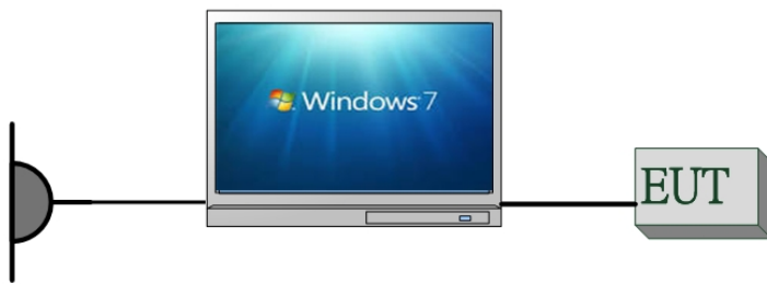
Fig. 2-1 Radiated & Conducted Emission Configuration
