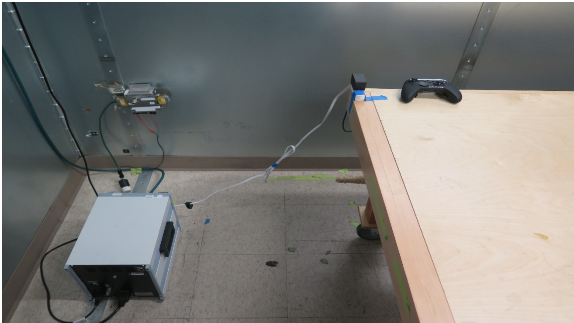
Figure 6 AC Line Conducted Emissions Test Setup -Front View
