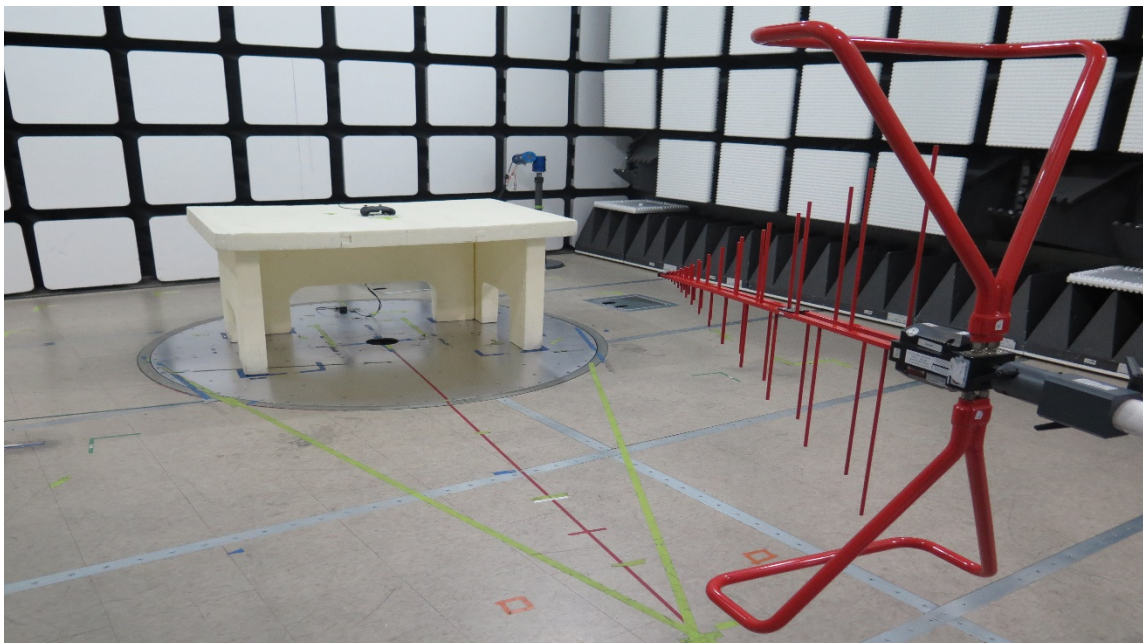
Figure 2 Radiated Spurious Emissions Test Setup (30M-1GHz)
