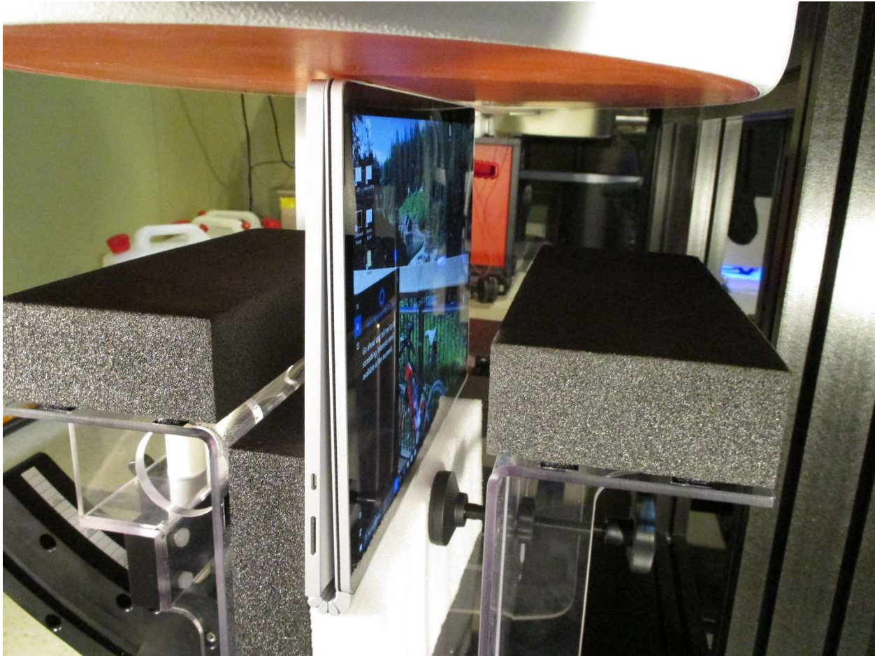
Photo 3 – Top Edge with Keyboard Folded Back 0mm
