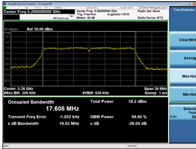
Plot 9-76. 26dB Emission Bandwidth and 99% OBW Chain A 802.11ac VHT 20 (CH. 52)
