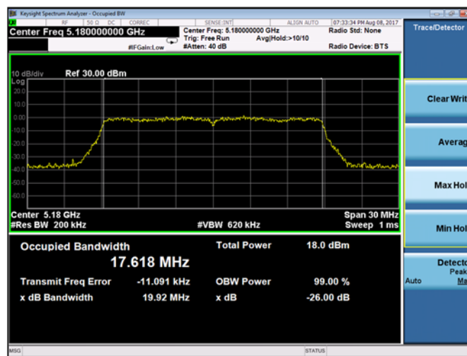
Plot 9-86. 26dB Emission Bandwidth and 99% OBW Chain B 802.11ac VHT 20 (CH. 36)
