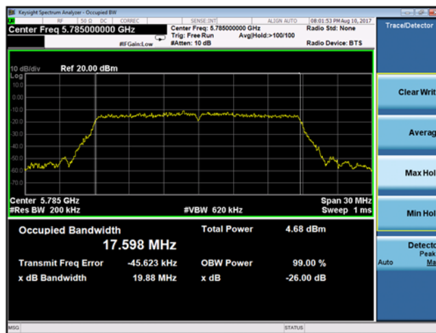
Plot 9-5. 26-dB Emission Bandwidth and 99% OBW 802.11n (Ch. 157)
