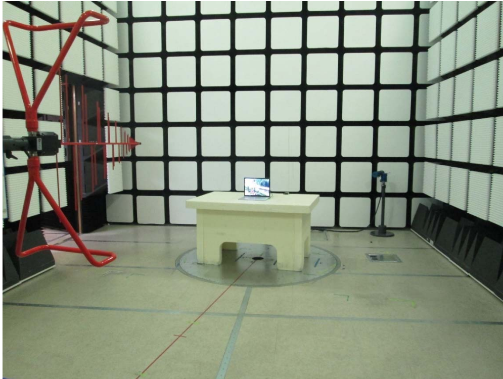
Fig.1 Radiated Spurious Emissions Test Setup (30MHz – 1GHz)
