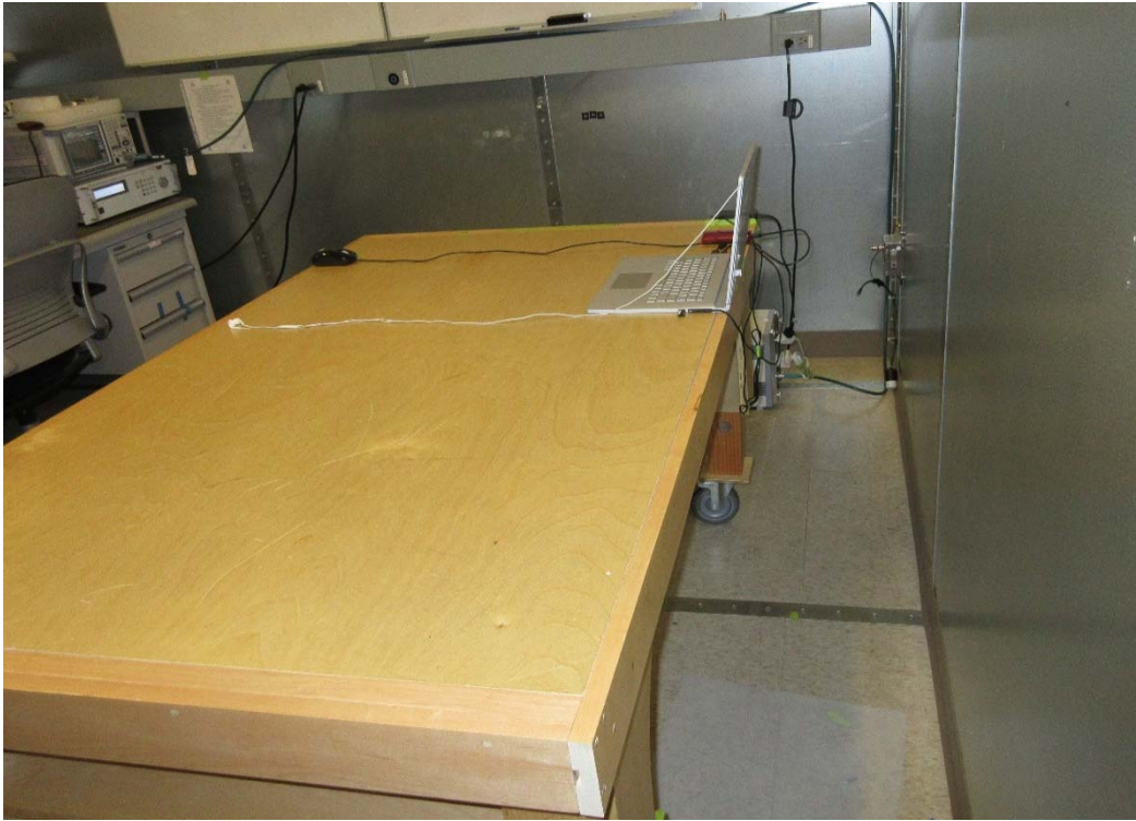
Fig.9 AC Line Conducted Emissions Measurements Test Setup- Side View
