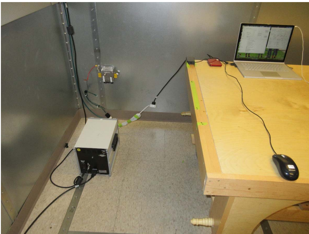
Fig.8 AC Line Conducted Emissions Measurements Test Setup- Front View 2
