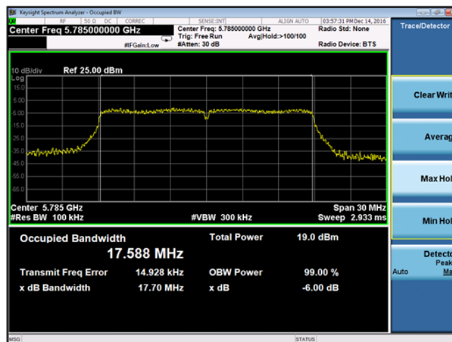
Plot 9-126. 6-dB Bandwidth Chain A 802.11n HT20 (Ch. 157)
