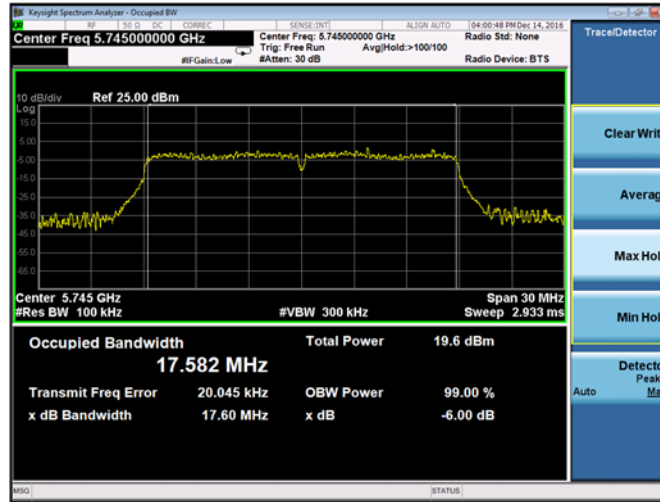
Plot 9-138. 6-dB Bandwidth Chain B 802.11ac VHT20 (Ch. 149)
