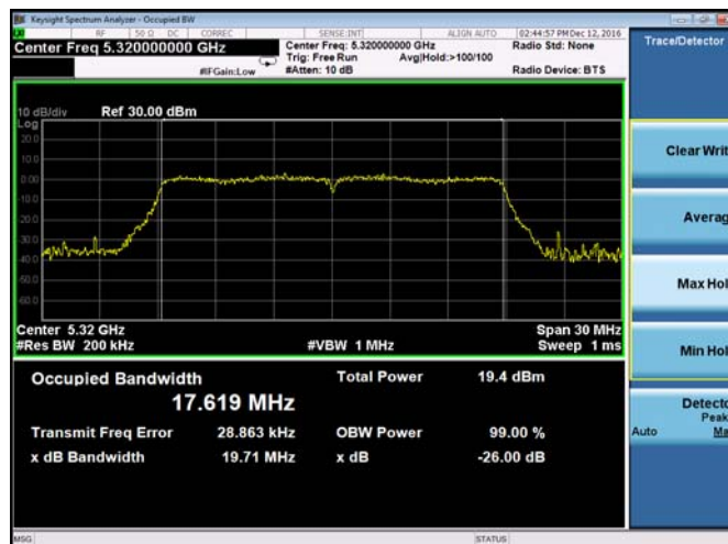
Plot 9-42. 26-dB Emission Bandwidth and 99% OBW Chain B 802.11n HT20 (Ch. 64)
