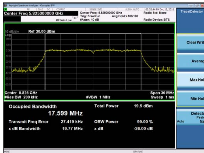
Plot 9-48. 26-dB Emission Bandwidth and 99% OBW Chain B 802.11n HT20 (Ch. 165)
