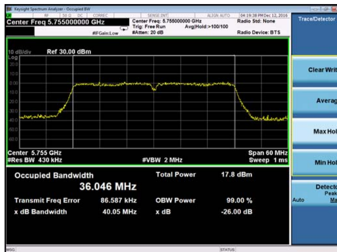
Plot 9-56. 26-dB Emission Bandwidth and 99% OBW Chain A 802.11n HT40 (Ch. 151)
