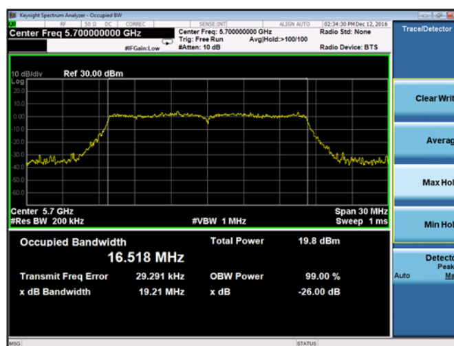
Plot 9-21. 26-dB Emission Bandwidth and 99% OBW Chain B 802.11a (Ch. 140)
