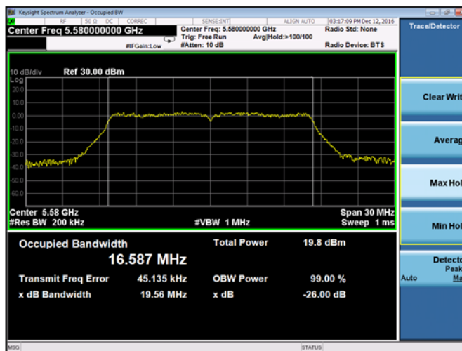
Plot 9-8. 26-dB Emission Bandwidth and 99% OBW Chain A 802.11a (Ch. 116)
