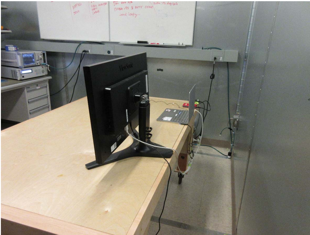
Fig.11 AC Line Conducted Emissions Measurements Test Setup- Side View
