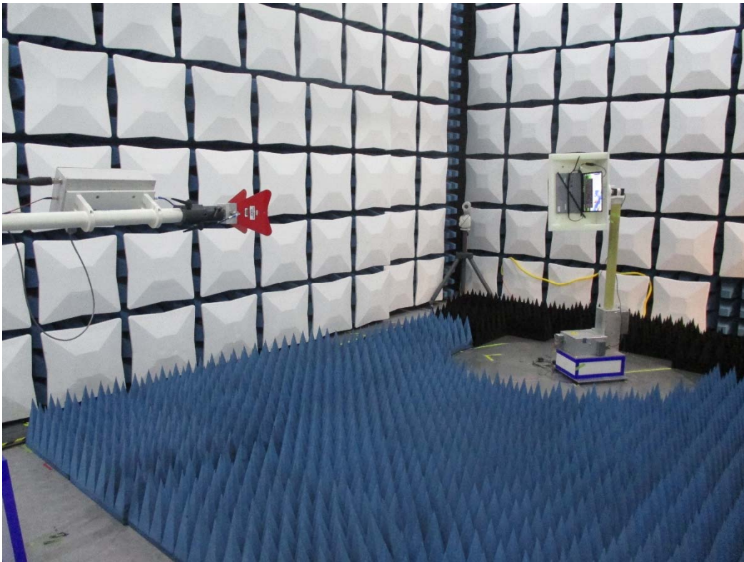
Fig 3. Radiated Spurious Emissions Test Setup (1-18 GHz) Test Site 2
