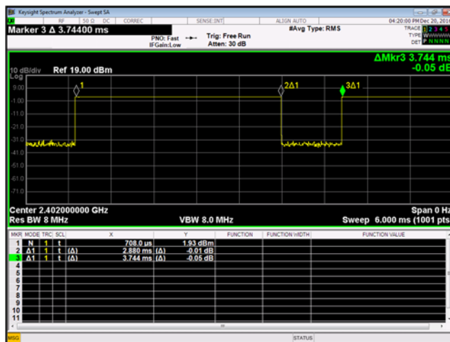
Plot 9-3. Duty Cycle (Ch. 0, 1-DH5)
