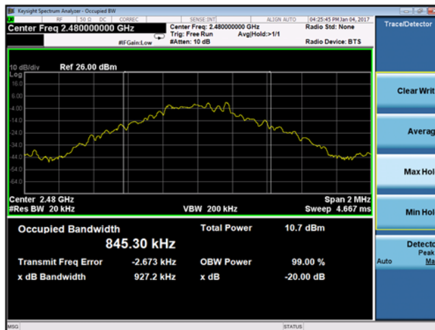
Plot 9-6. 20dB Bandwidth (Ch. 78, 1-DH5)
