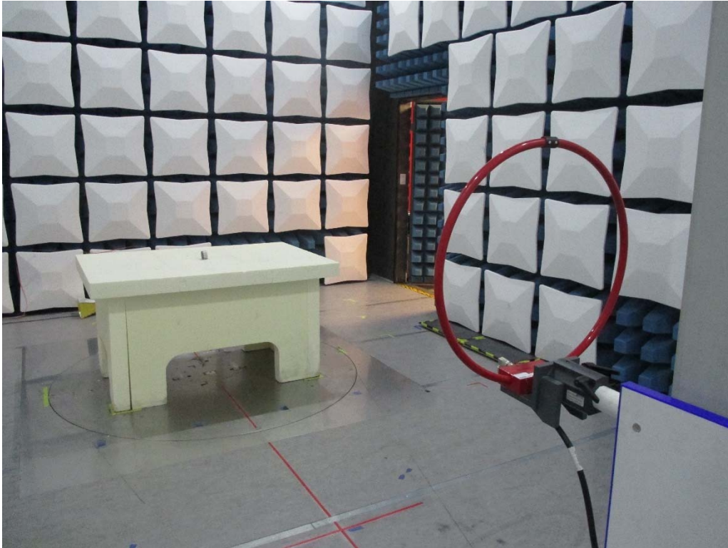
Figure 1. Radiated Spurious Emissions Test Setup (9 kHz – 30 MHz)
