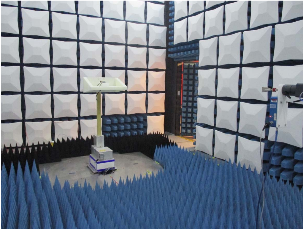
Figure 5. Radiated Spurious Emissions Test Setup (18-26.5GHz)
