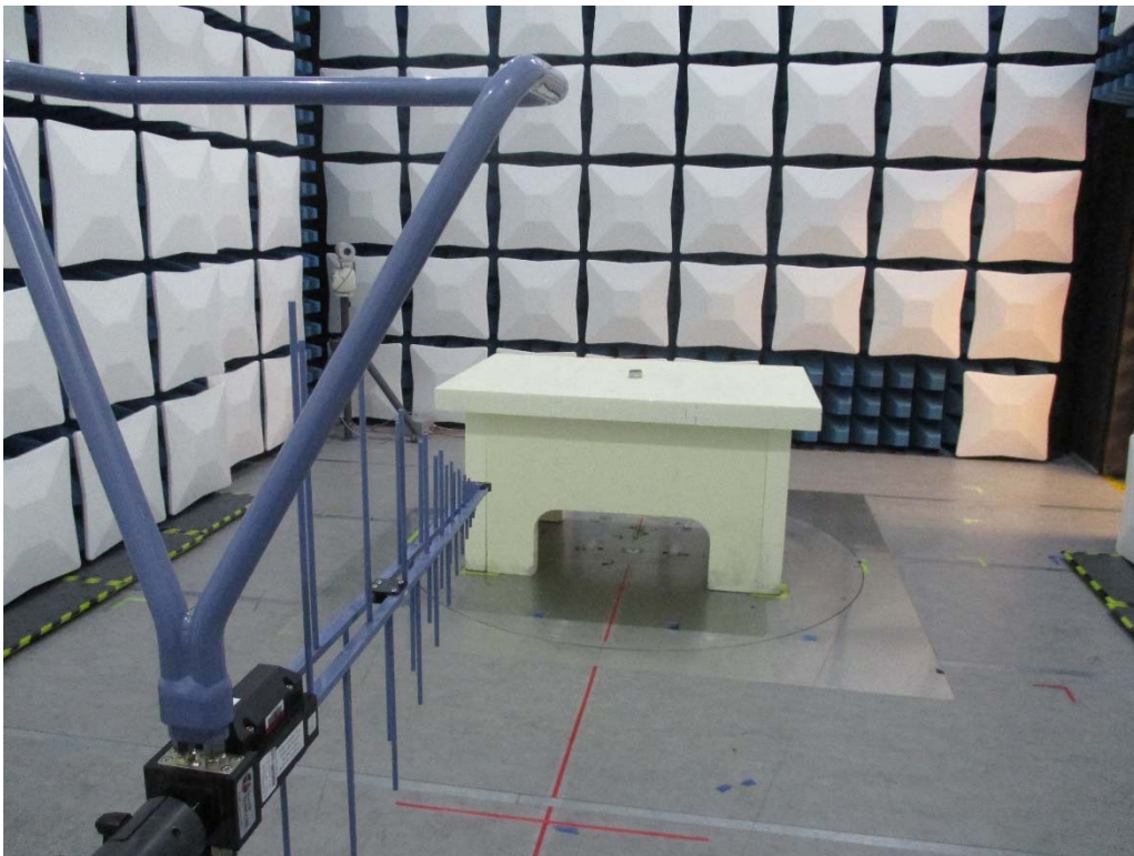
Figure 2. Radiated Spurious Emissions Test Setup (30MHz – 1GHz)
