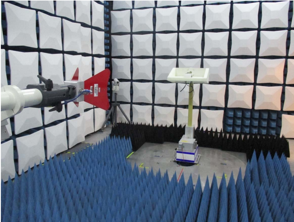
Figure 3. Radiated Spurious Emissions Test Setup (1-18 GHz) Test Site 1
