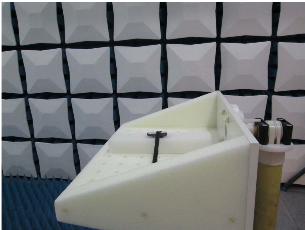
Fig 4. Radiated Spurious Emissions Test Setup (1-18 GHz) EUT Setup
