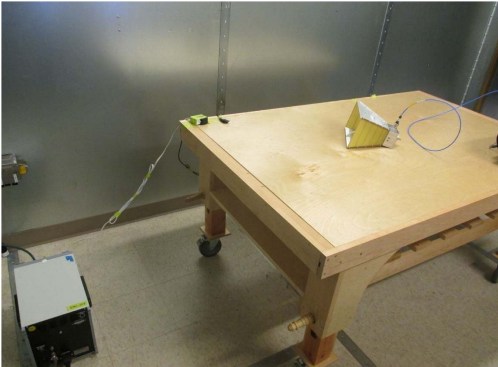
Fig. 8 AC Line Conducted Emissions Test Setup 2 (Side of EUT with 80cm LISN spacing)
