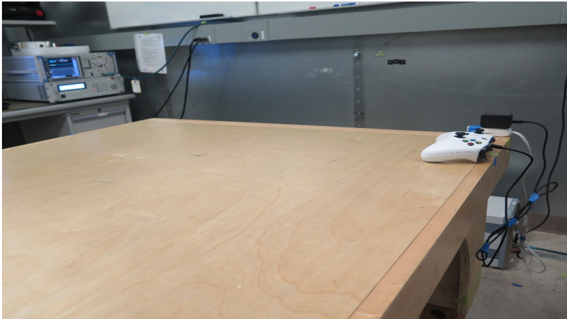
Figure 7 AC Line Conducted Emissions Test Setup -Side View
