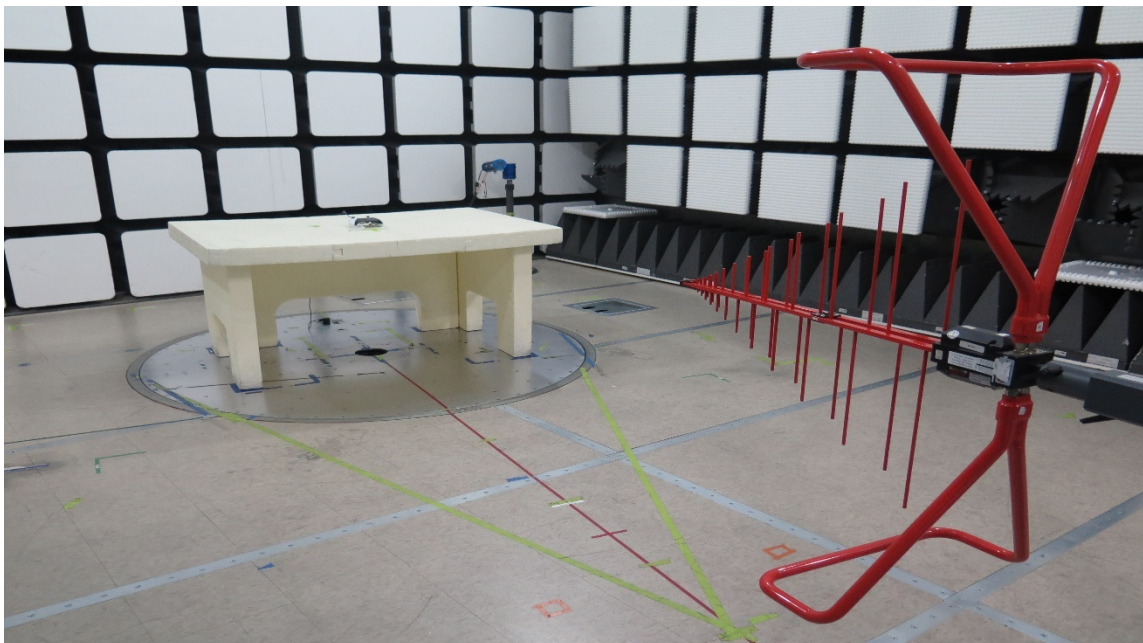
Figure 2 Radiated Spurious Emissions Test Setup (30M-1GHz)
