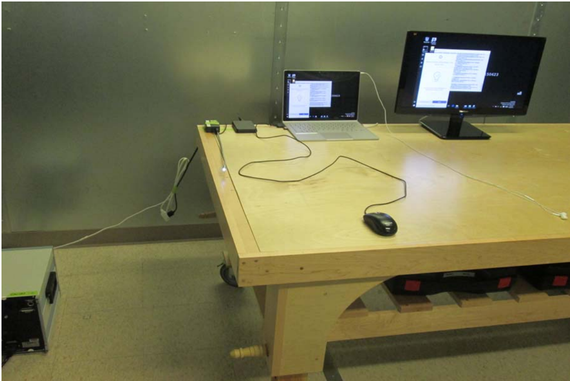
Fig.7 AC Line Conducted Emissions Measurements Test Setup
