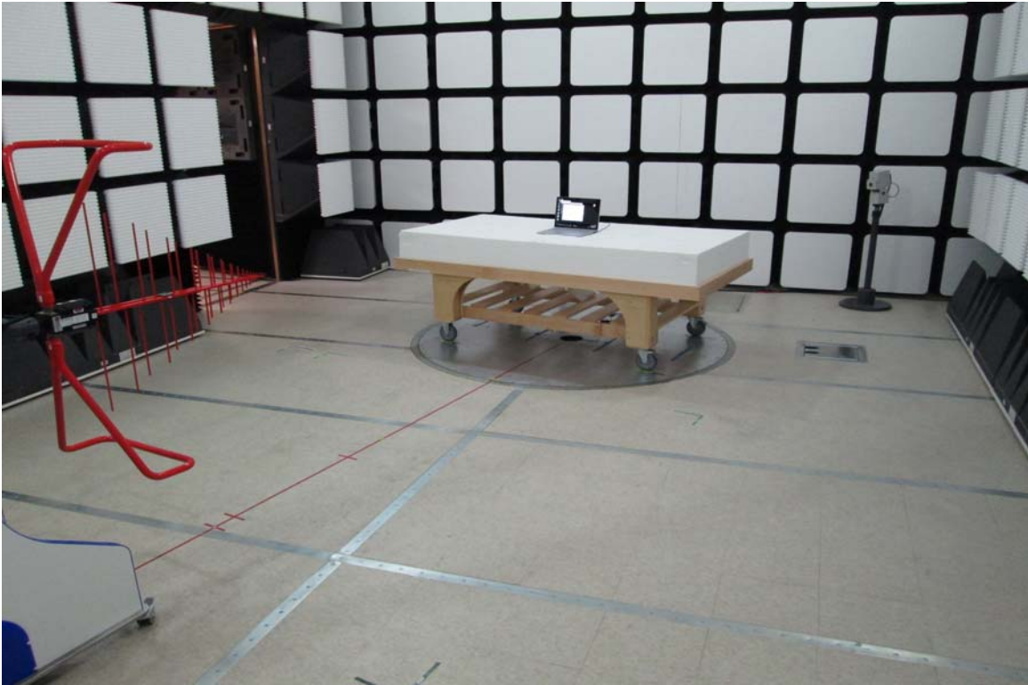
Fig.1 Radiated Spurious Emissions Test Setup (30MHz – 1GHz)
