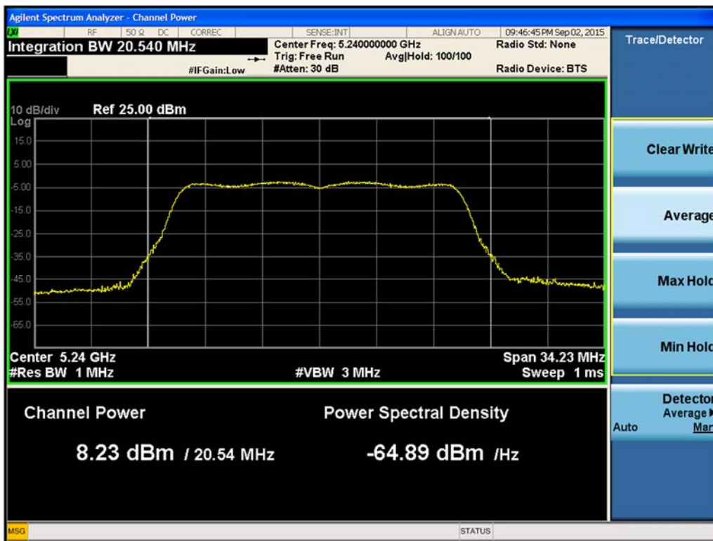
Figure 316. Maximum Conducted Output Power Chain A 802.11n HT20 (Ch. 48)
