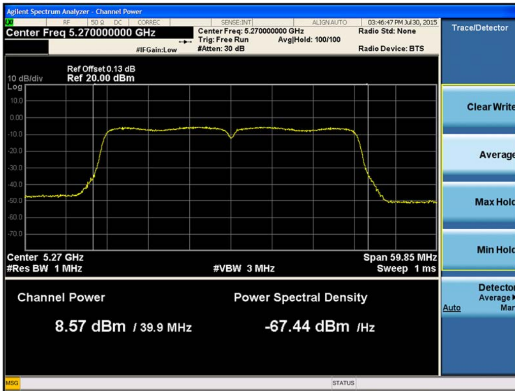
Figure 364. Maximum Conducted Output Power Chain A 802.11n HT40 (Ch. 54)
