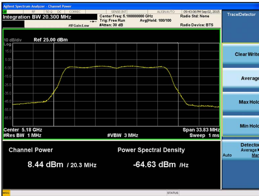
Figure 290. Maximum Conducted Output Power Chain A 802.11a (Ch. 36)
