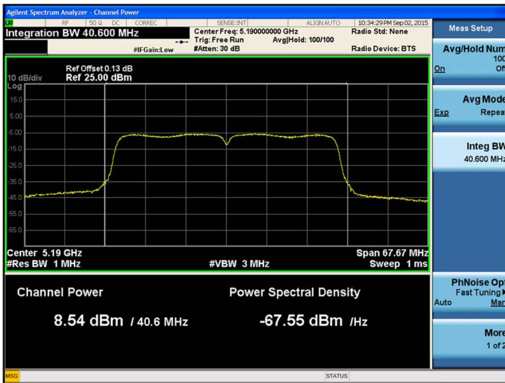
Figure 362. Maximum Conducted Output Power Chain A 802.11n HT40 (Ch. 38)
