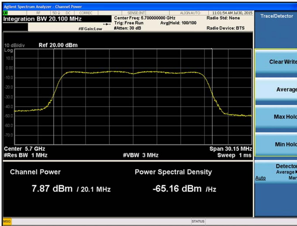
Figure 358. Maximum Conducted Output Power Chain B 802.11ac VHT20 (Ch. 140)
