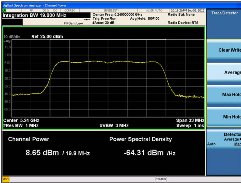
Figure 352. Maximum Conducted Output Power Chain B 802.11ac VHT20 (Ch. 48)
