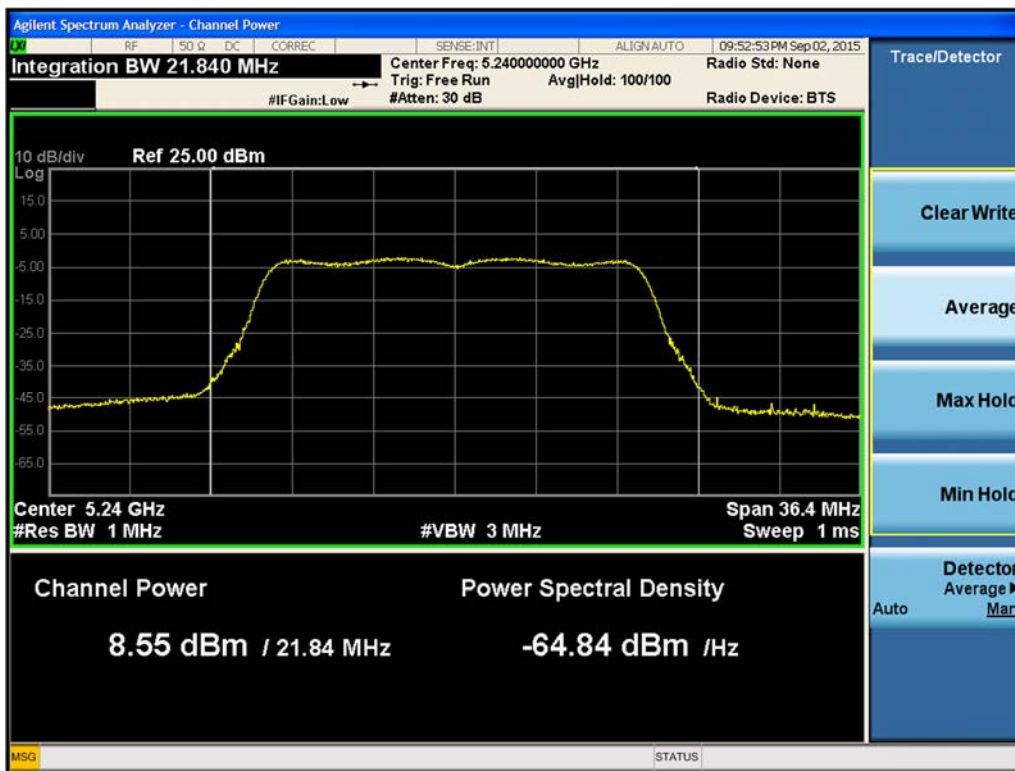
Figure 328. Maximum Conducted Output Power Chain B 802.11n HT20 (Ch. 48)
