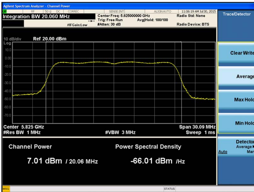
Figure 361. Maximum Conducted Output Power Chain B 802.11ac VHT20 (Ch. 165)
