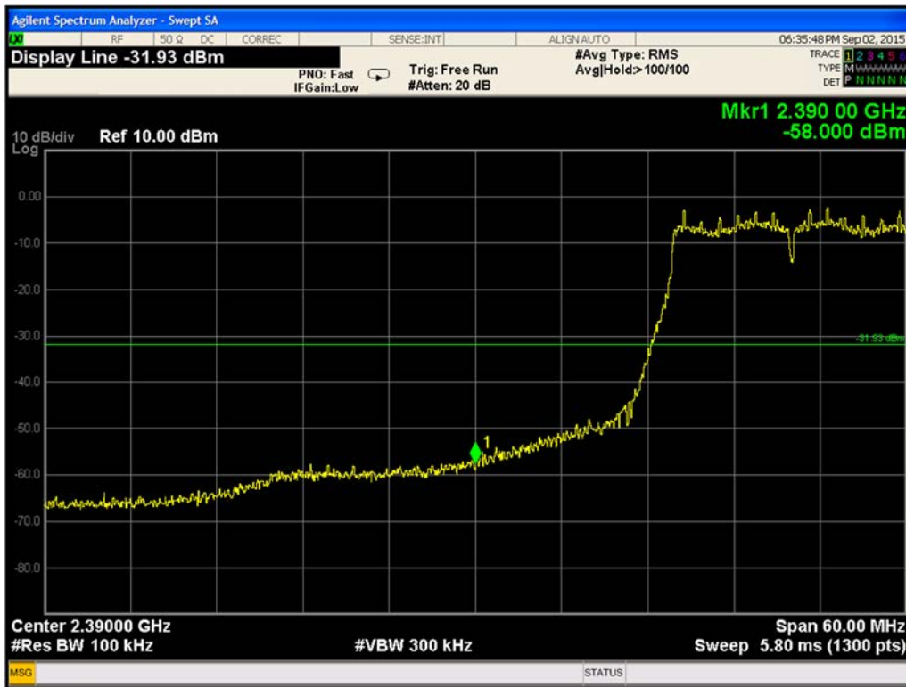
Plot 9-172. Conducted-Low Band Edge 802.11g Path B (Ch. 1)
