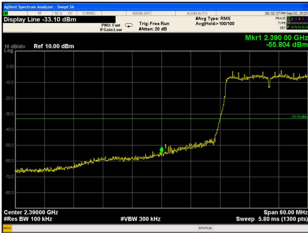
Plot 9-170. Conducted-Low Band Edge 802.11n Path A (Ch. 1)
