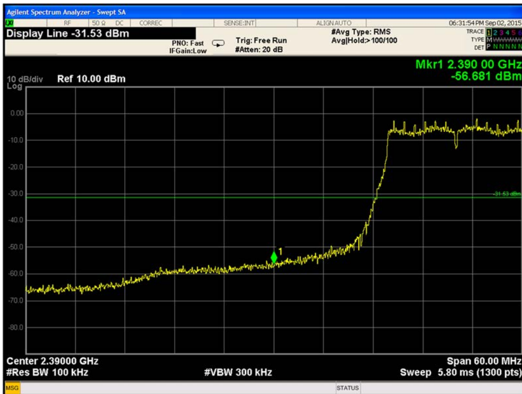
Plot 9-169. Conducted-Low Band Edge 802.11g Path A (Ch. 1)
