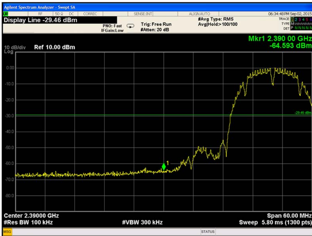
Plot 9-171. Conducted-Low Band Edge 802.11b Path B (Ch. 1)
