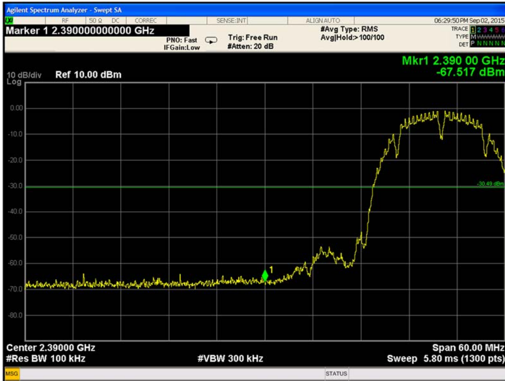
Plot 9-168. Conducted-Low Band Edge 802.11b Path A (Ch. 1)
