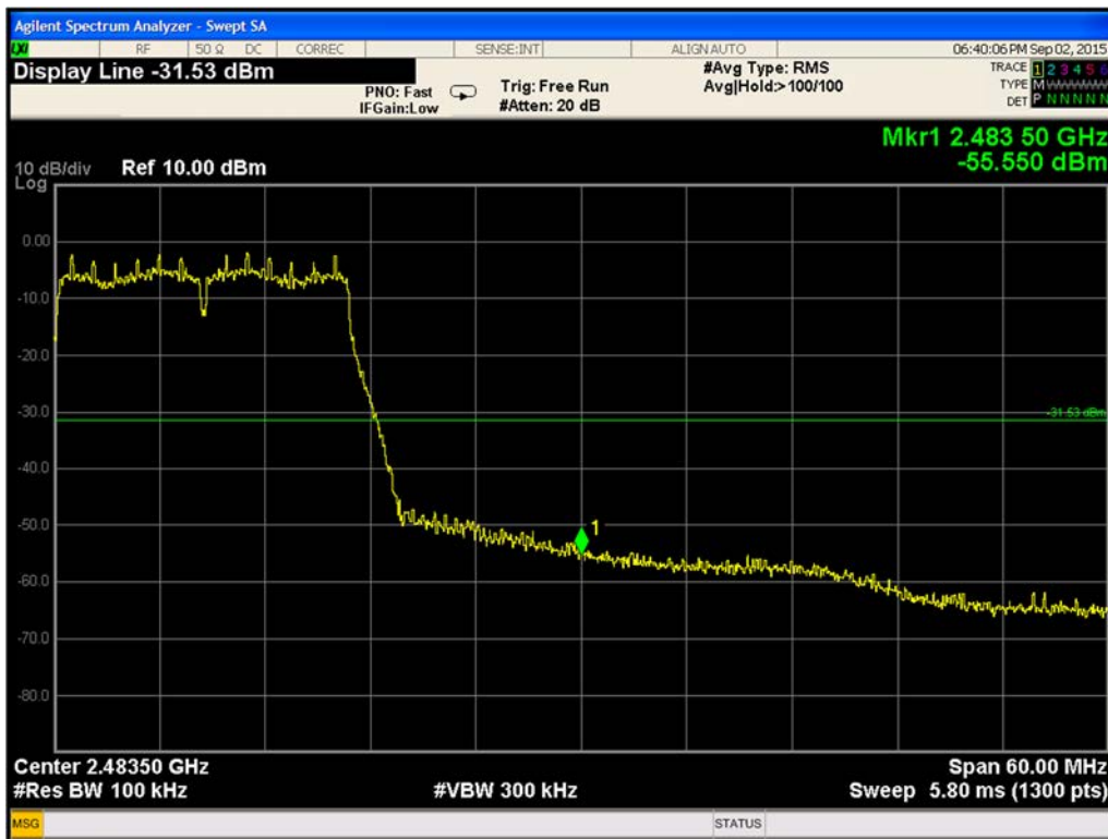
Plot 9-175. Conducted-Upper Band Edge 802.11g Path A (Ch. 11)
