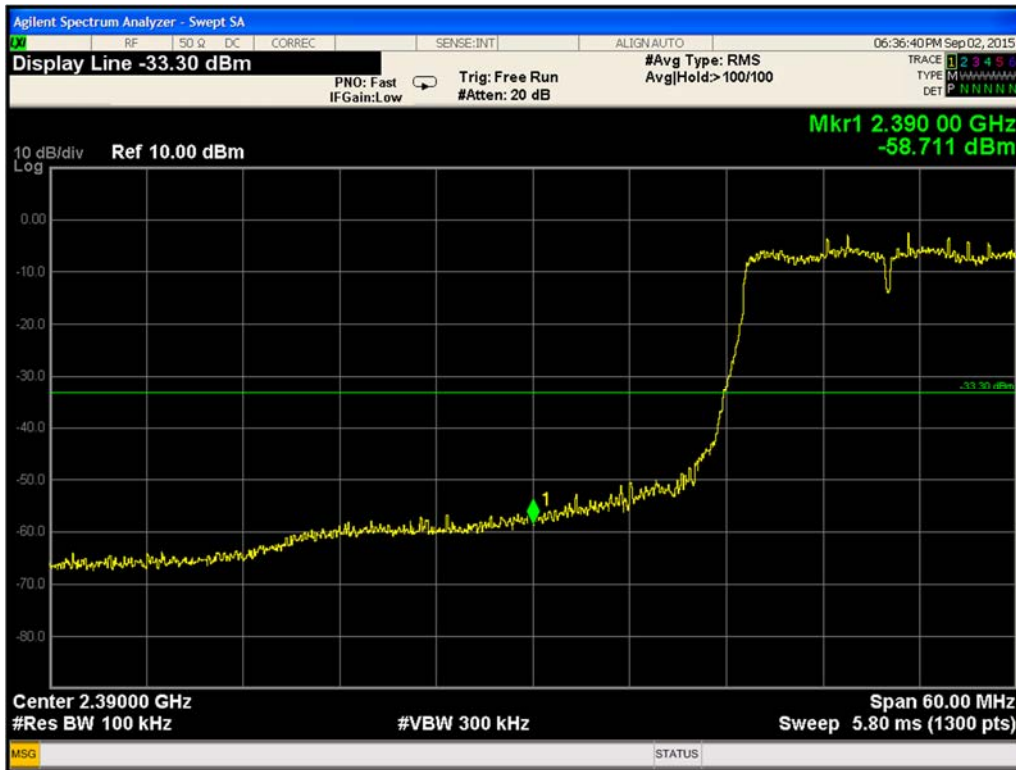
Plot 9-173. Conducted-Low Band Edge 802.11n Path B (Ch. 1)
