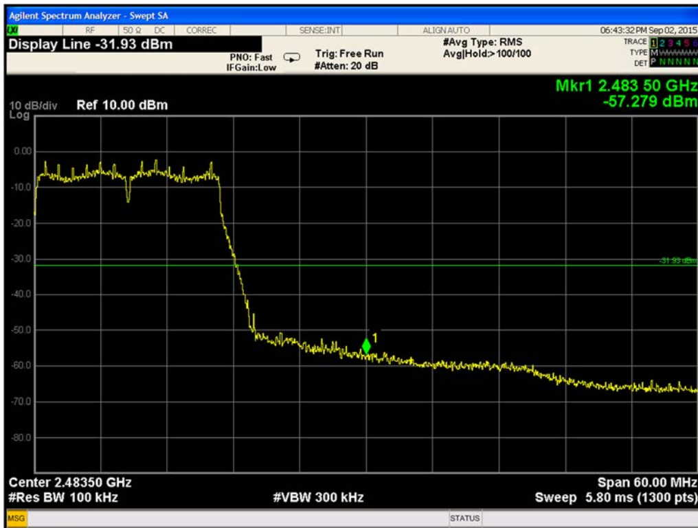
Plot 9-178. Conducted-Upper Band Edge 802.11g Path B (Ch. 11)
