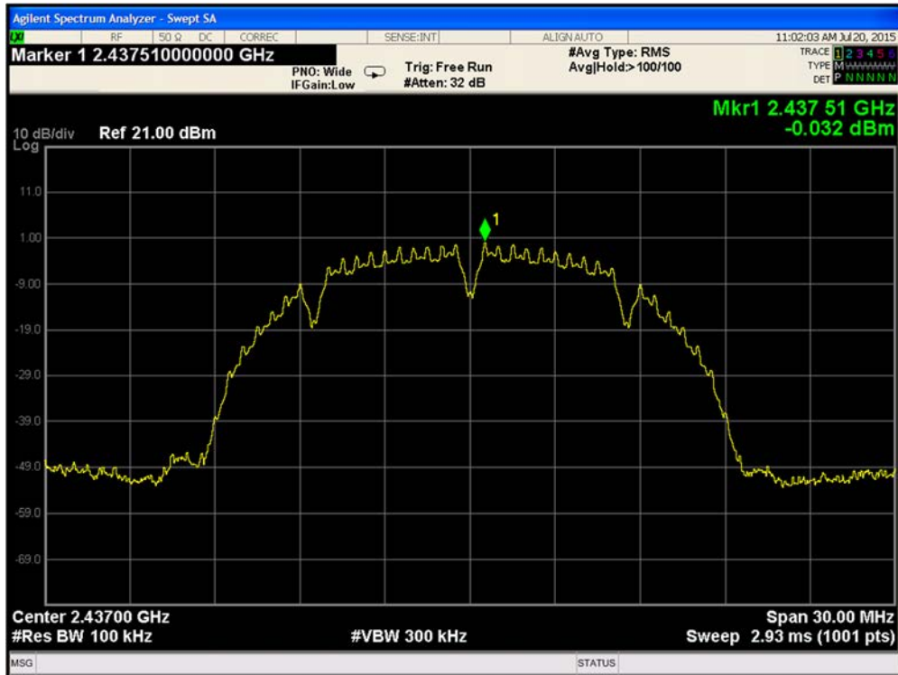
Plot 9-100. Reference Level Measurement 802.11b Path A Ch6
