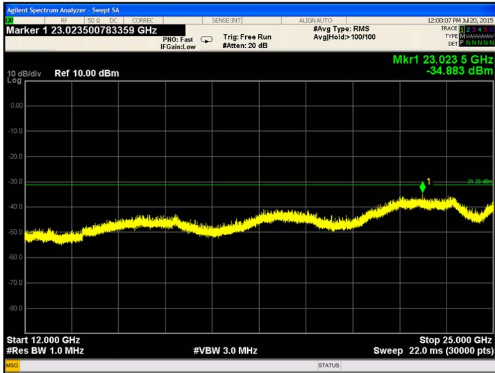
Plot 9-113. Conducted Spurious Emissions 802.11g 12GHz – 25 GHz Path A CH11
