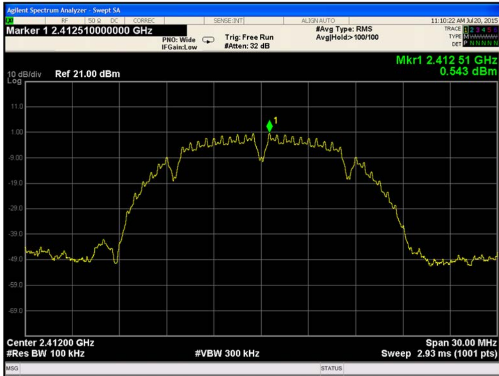
Plot 9-123. Reference Level Measurement 802.11b Path B Ch1
