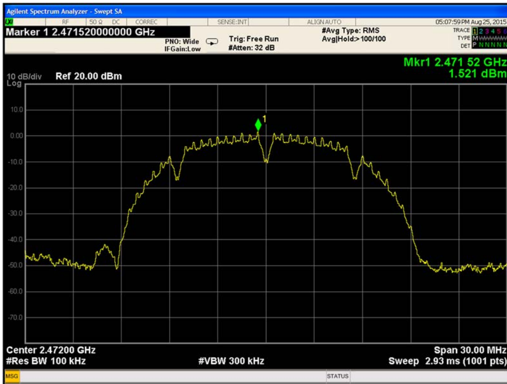
Plot 9-159. Reference Level Measurement 802.11b Path B Ch13
