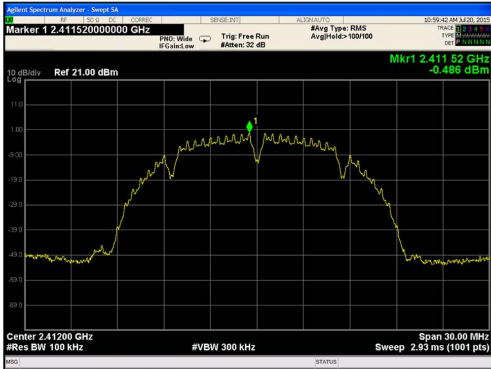
Plot 9-97. Reference Level Measurement 802.11b Path A Ch1
