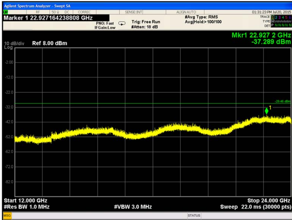
Plot 9-125. Conducted Spurious Emissions 802.11b 12GHz – 25 GHz Path B CH1
