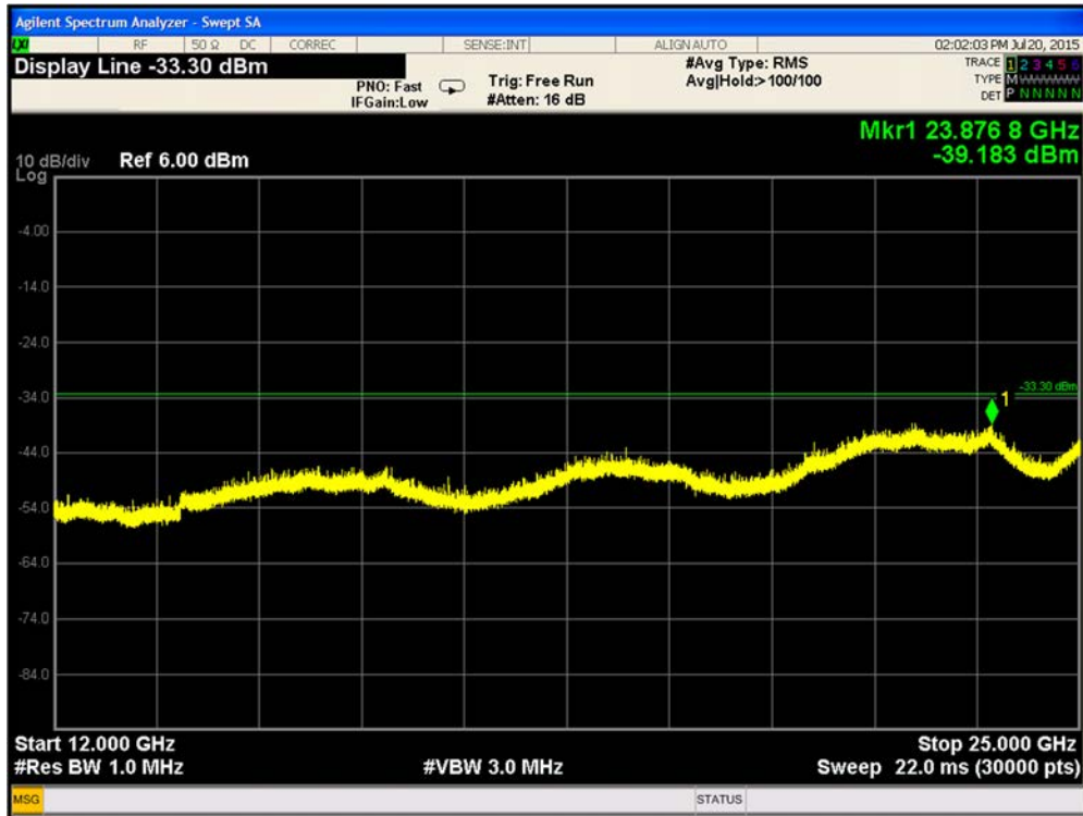
Plot 9-143. Conducted Spurious Emissions 802.11n 12GHz – 25 GHz Path B CH1
