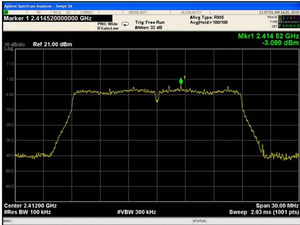
Plot 9-114. Reference Level Measurement 802.11n Path A Ch1
