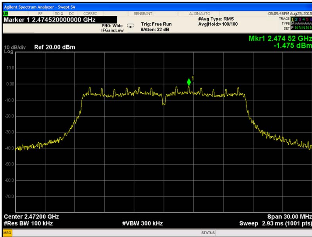
Plot 9-162. Reference Level Measurement 802.11g Path B Ch13
