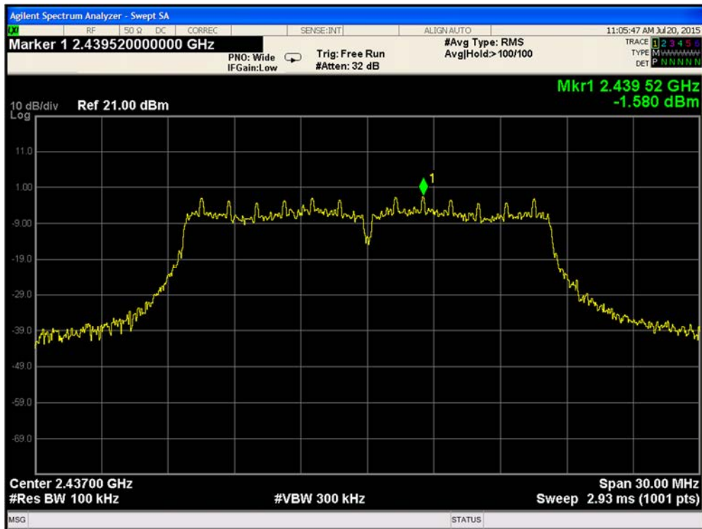
Plot 9-109. Reference Level Measurement 802.11g Path A Ch6
