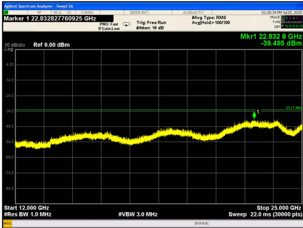
Plot 9-122. Conducted Spurious Emissions 802.11n 12GHz – 25 GHz Path A CH11
