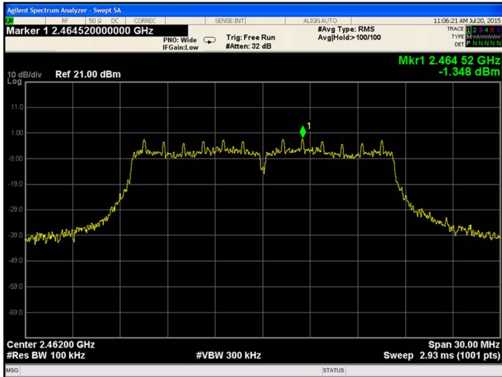
Plot 9-111. Reference Level Measurement 802.11g Path A Ch11
