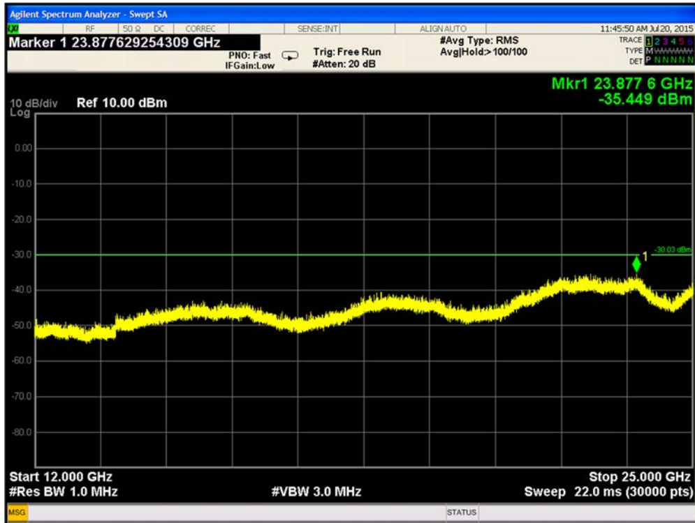
Plot 9-102. Conducted Spurious Emissions 802.11b 12GHz – 25 GHz Path A CH6
