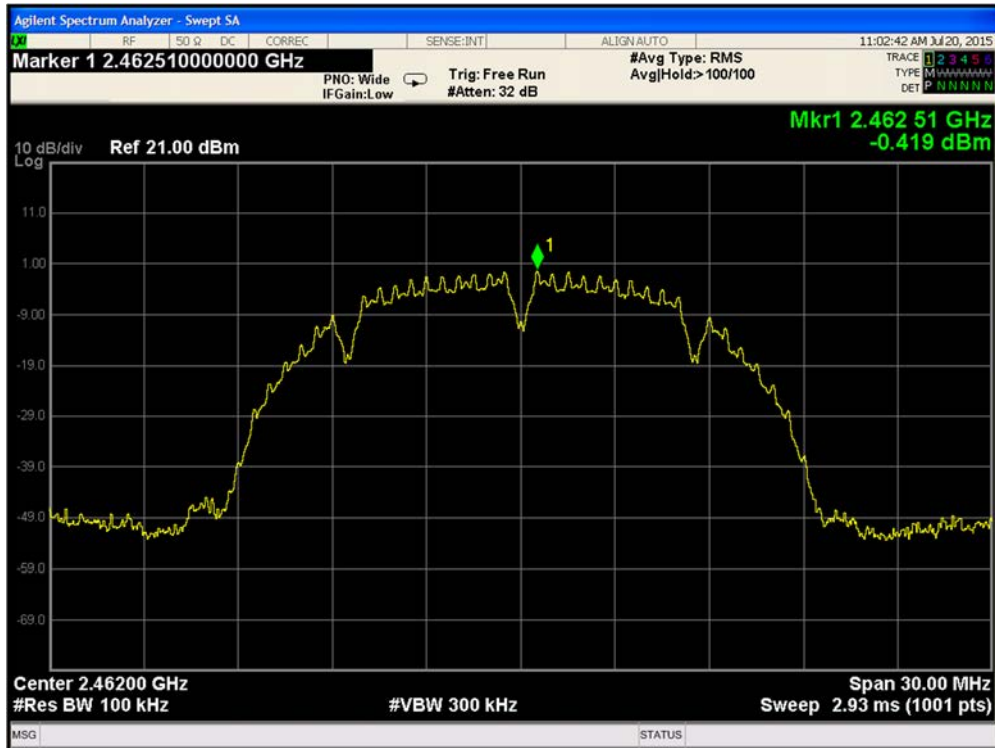
Plot 9-103. Reference Level Measurement 802.11b Path A Ch11
