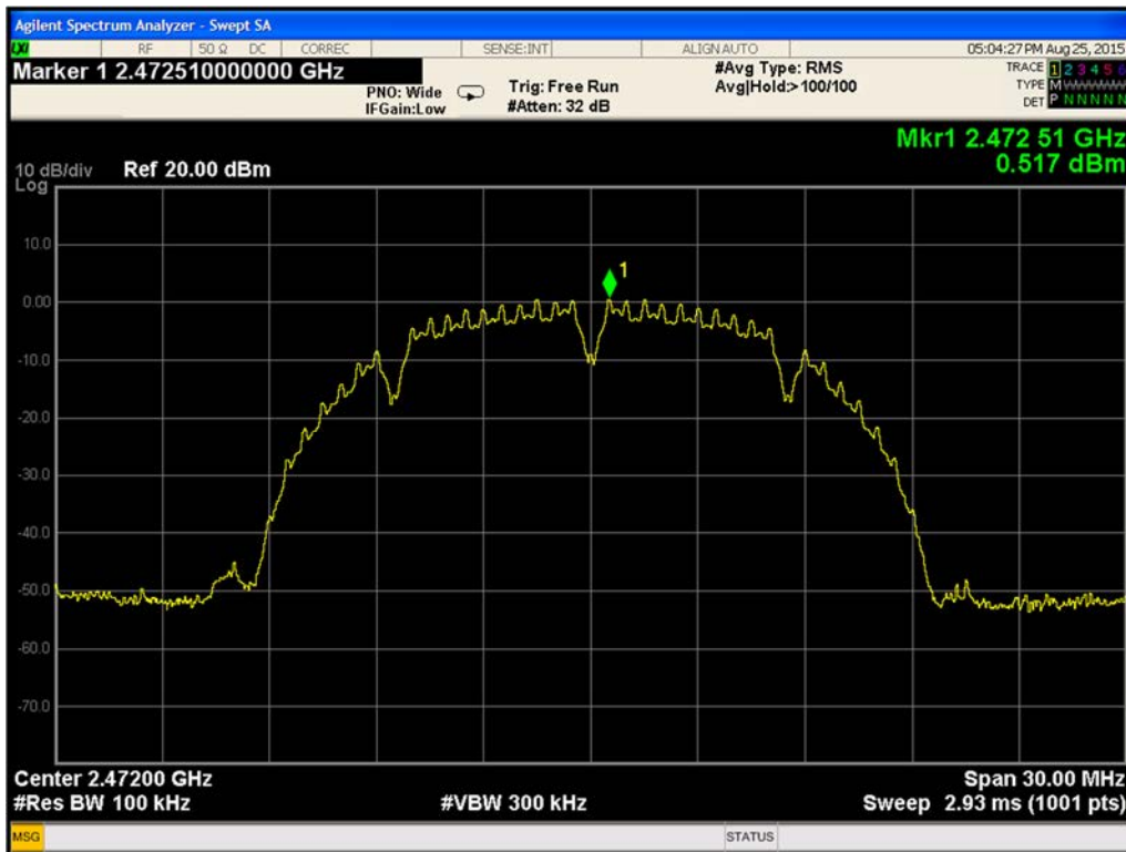
Plot 9-150. Reference Level Measurement 802.11b Path A Ch13
