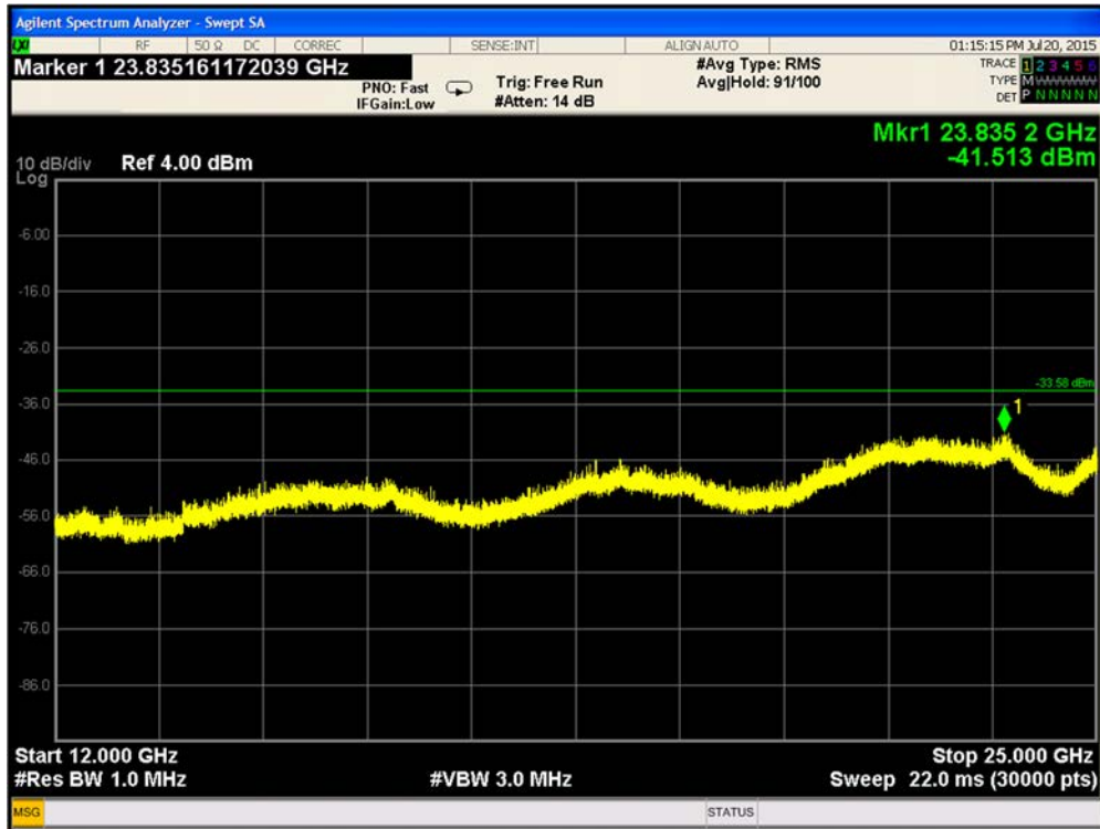
Plot 9-119. Conducted Spurious Emissions 802.11n 12GHz – 25 GHz Path A CH6
