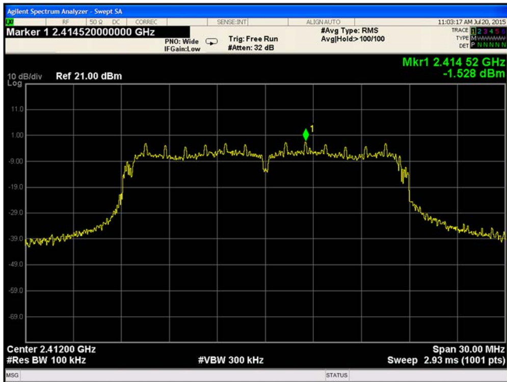
Plot 9-106. Reference Level Measurement 802.11g Path A Ch1
