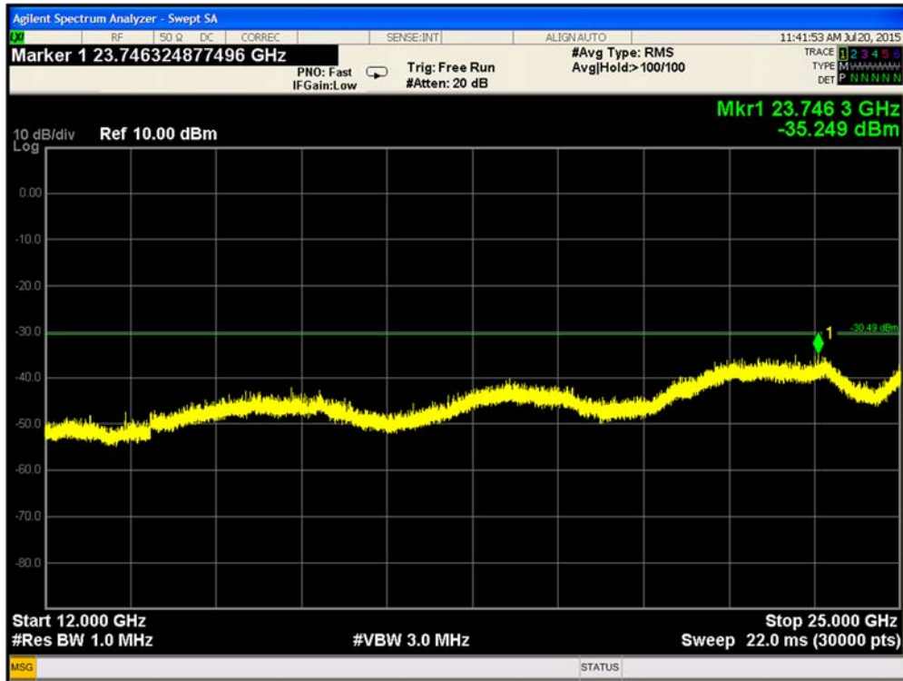
Plot 9-99. Conducted Spurious Emissions 802.11b 12GHz – 25 GHz Path A CH1
