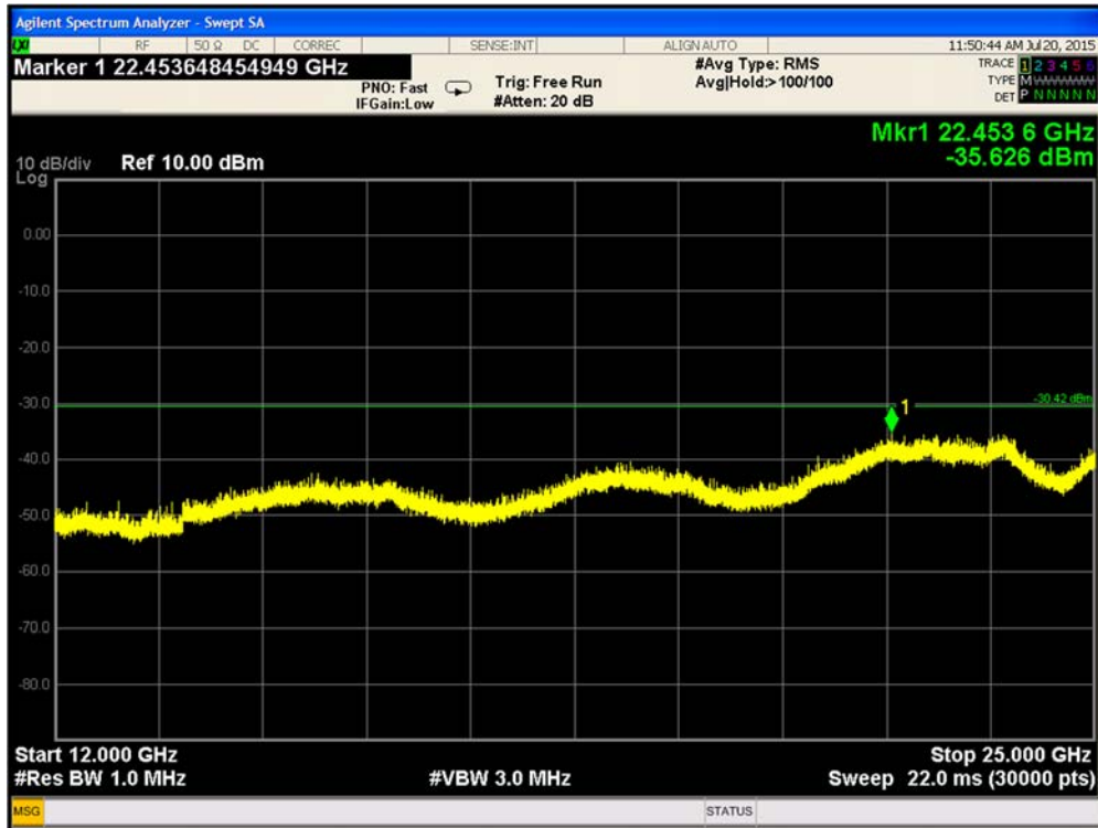
Plot 9-105. Conducted Spurious Emissions 802.11b 12GHz – 25 GHz Path A CH11
