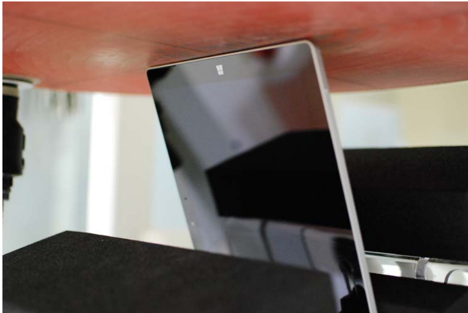
SAR Test Setup Photo 10: Right Edge Tilt at 0.0 cm
