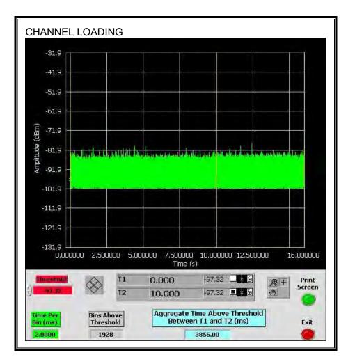
The level of traffic loading on the channel by the EUT is 38.56%
