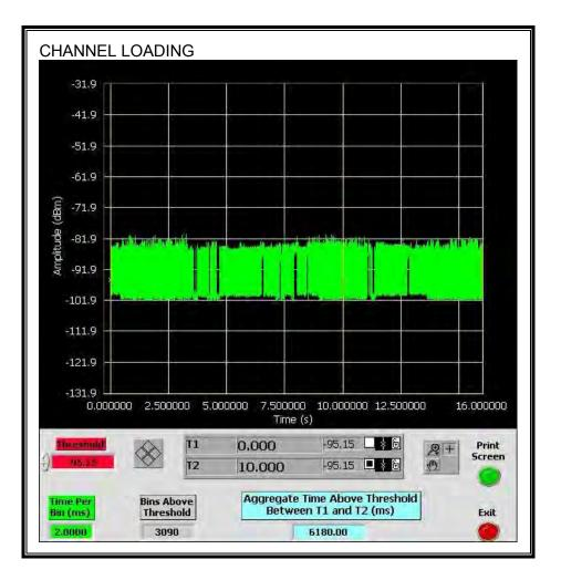
The level of traffic loading on the channel by the EUT is 61.8%
