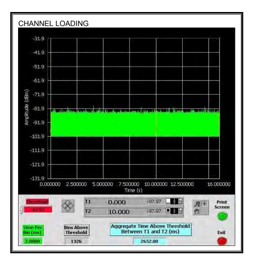
The level of traffic loading on the channel by the EUT is 26.52%
