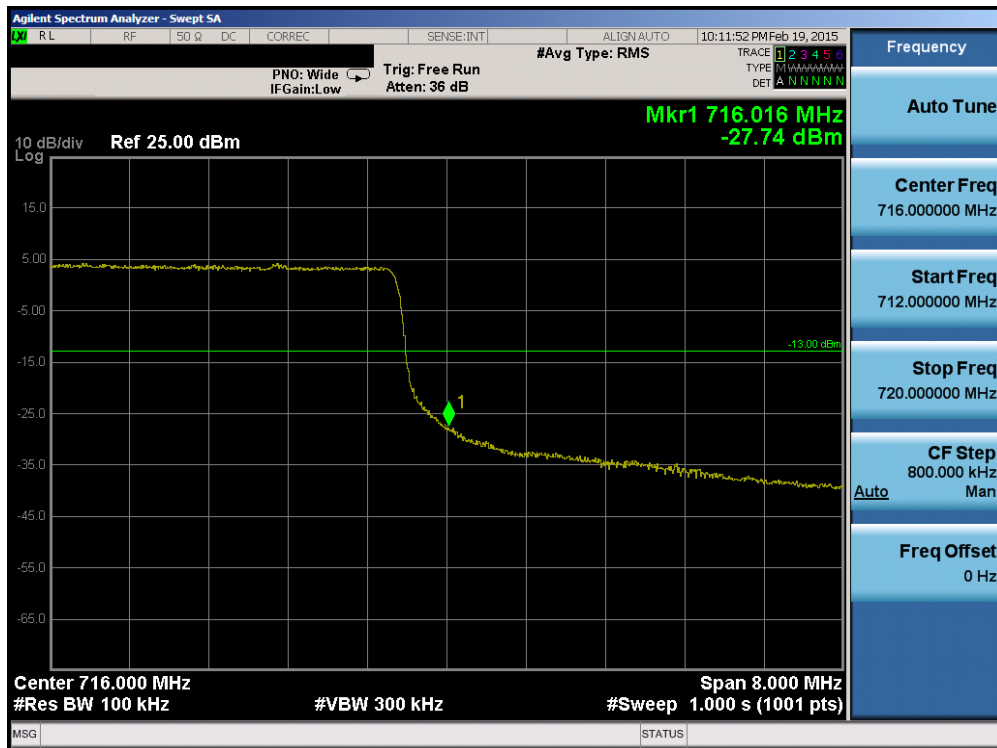
Plot 6-91. Upper Band Edge Plot (Band 17 – 10.0MHz QPSK – RB Size 50)
