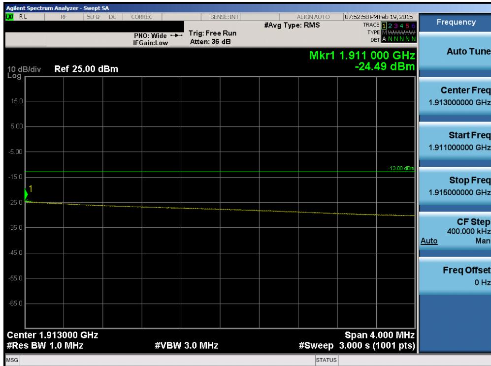
Plot 6-159. Upper Extended Band Edge Plot (Band 2 – 15.0MHz QPSK – RB Size 75)
