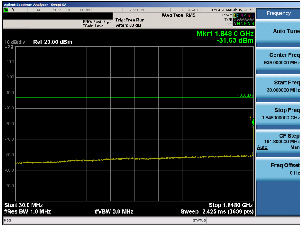
Plot 6-77. Conducted Spurious Plot (Band 2 – 10.0MHz QPSK – RB Size 1, RB Offset 0– Low Channel)
