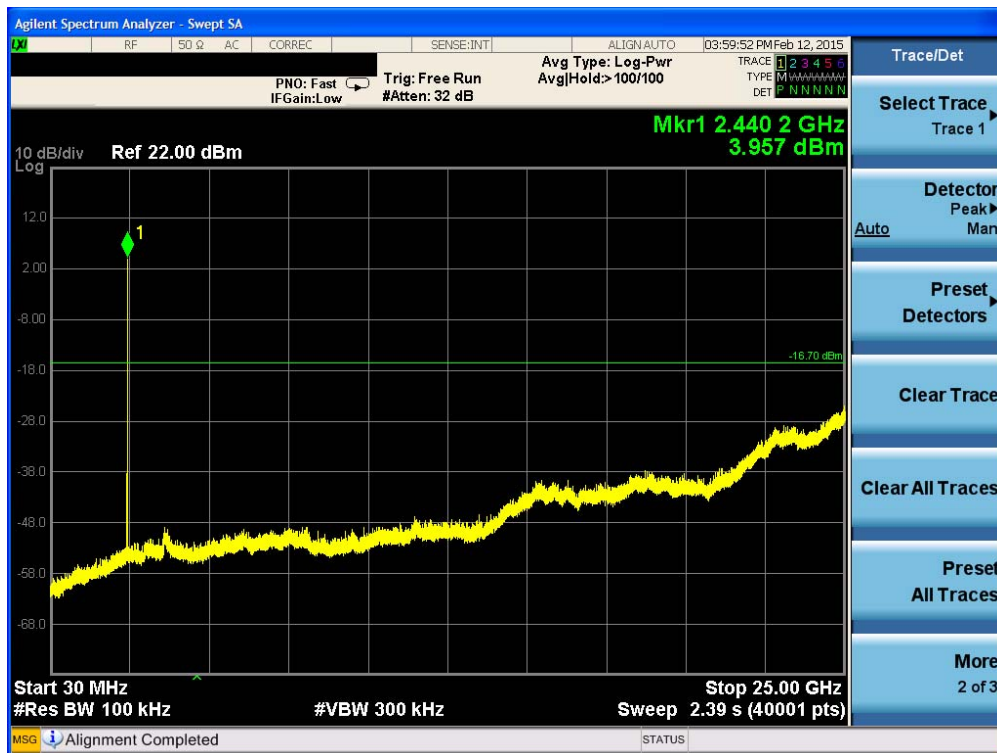
Plot 9-14. Conducted Spurious Emissions (Ch. 19)
