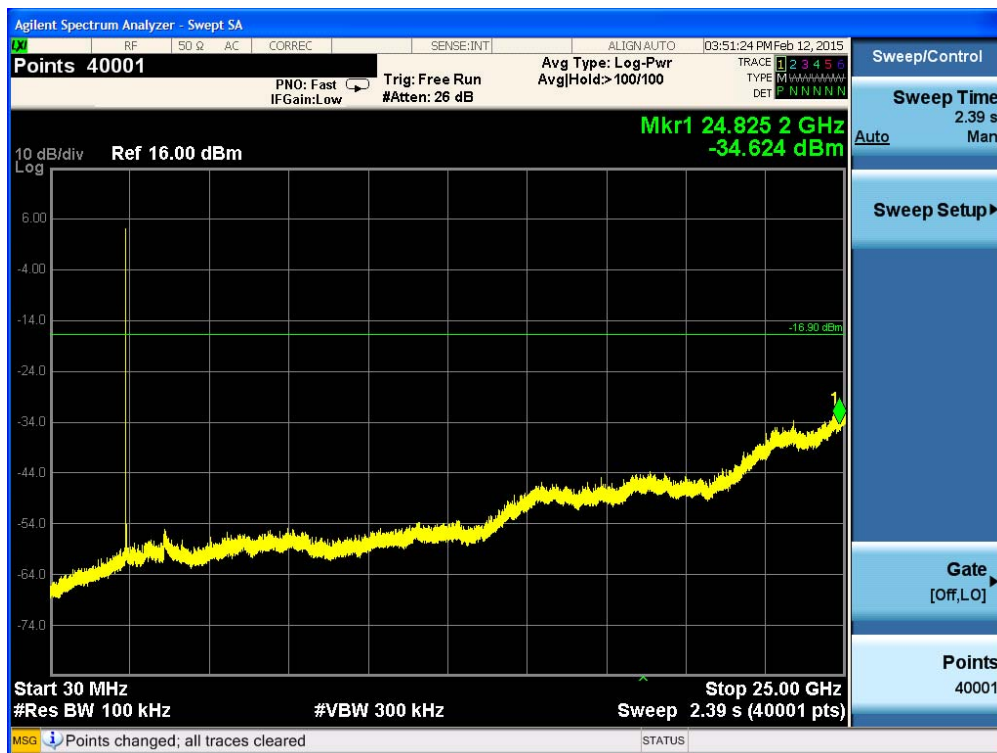
Plot 9-13. Conducted Spurious Emissions (Ch. 0)
