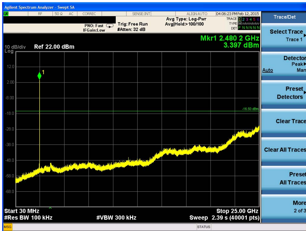
Plot 9-15. Conducted Spurious Emissions (Ch. 39)
