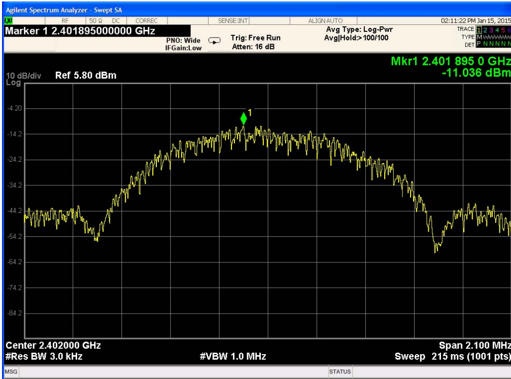
Plot 9-10. Power Spectral Density (Ch. 0)
