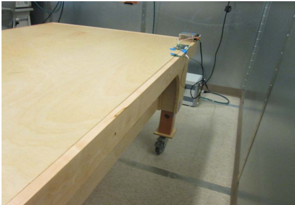
Fig.9 AC Line Conducted Emissions Measurements Test Setup – Back
