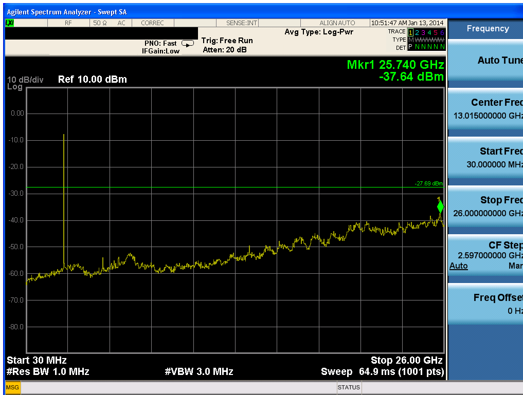
Plot 9-15. Conducted Spurious Emissions (Ch. 0)
