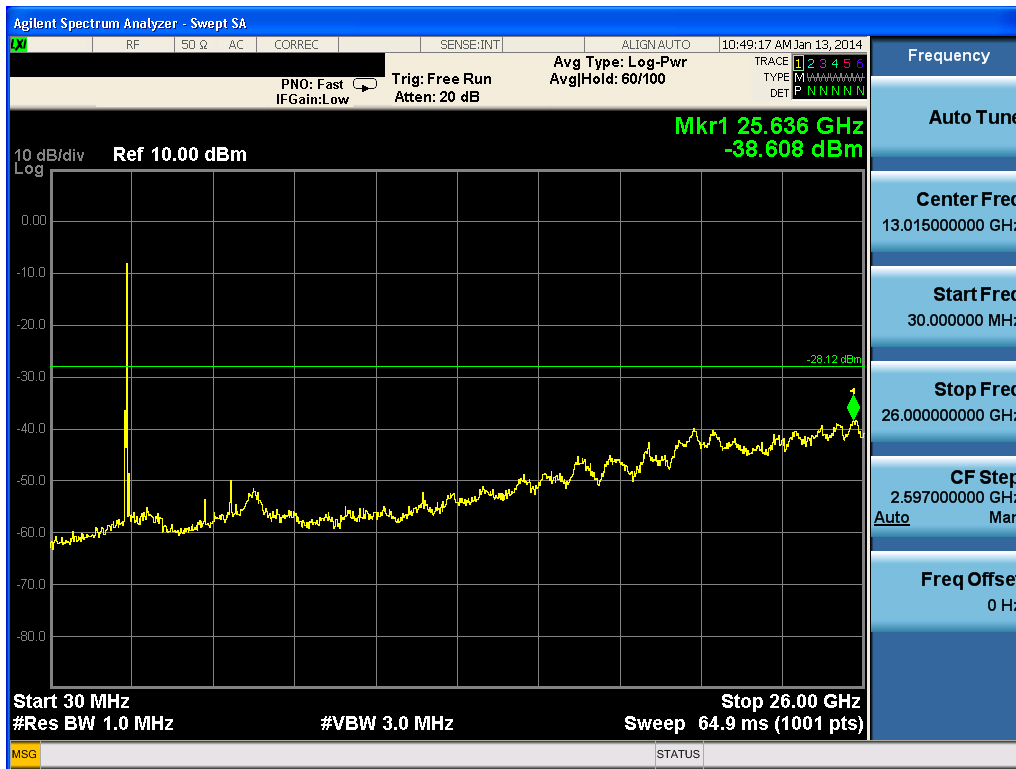
Plot 9-17. Conducted Spurious Emissions (Ch. 39)
