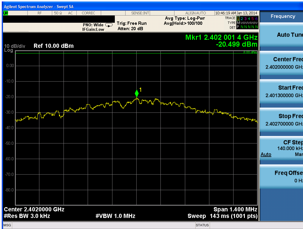
Plot 9-10. Power Spectral Density (Ch. 0)
