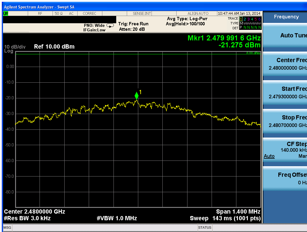
Plot 9-12. Power Spectral Density (Ch. 39)
