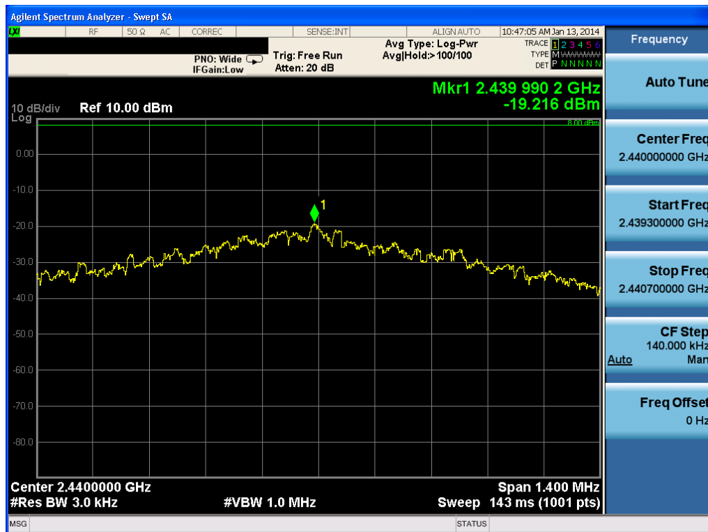
Plot 9-11. Power Spectral Density (Ch. 19)
