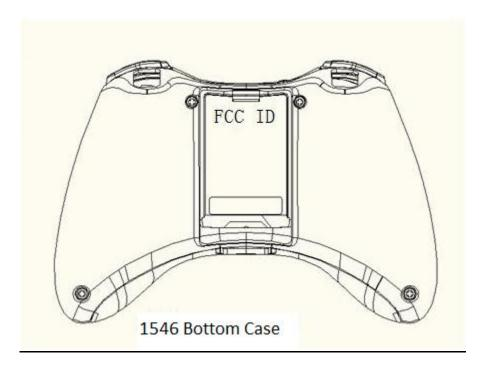
Note: Location indicated above is inside battery compartment. It is not on the removable battery cover.
