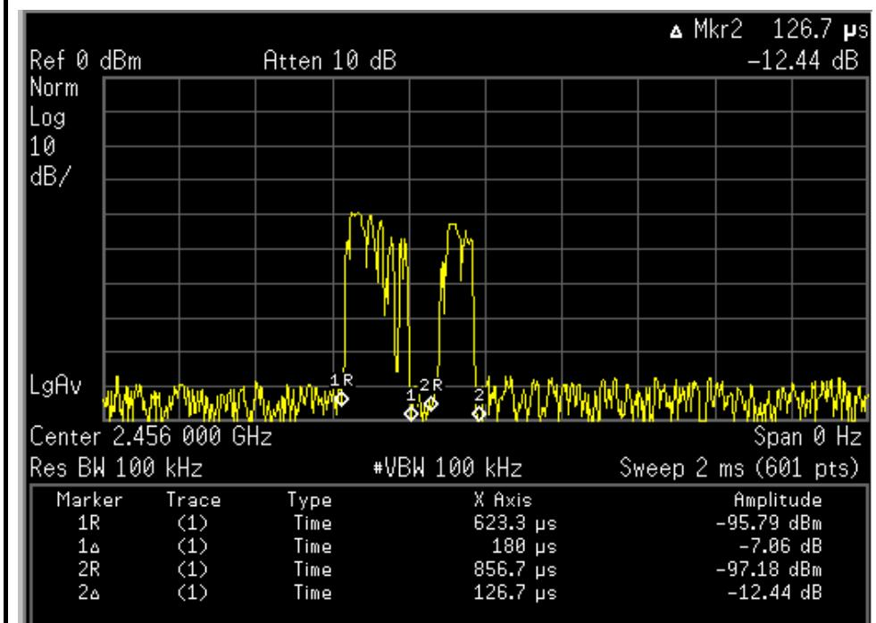
Duty cycle=  $\frac{180+126.7\mu s}{8 \text{ ms}}$  x100% = 3.83%
