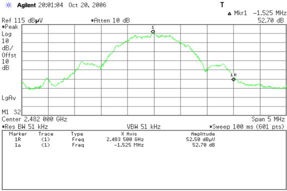
Delta marker at 1% of span = 52.70dB
