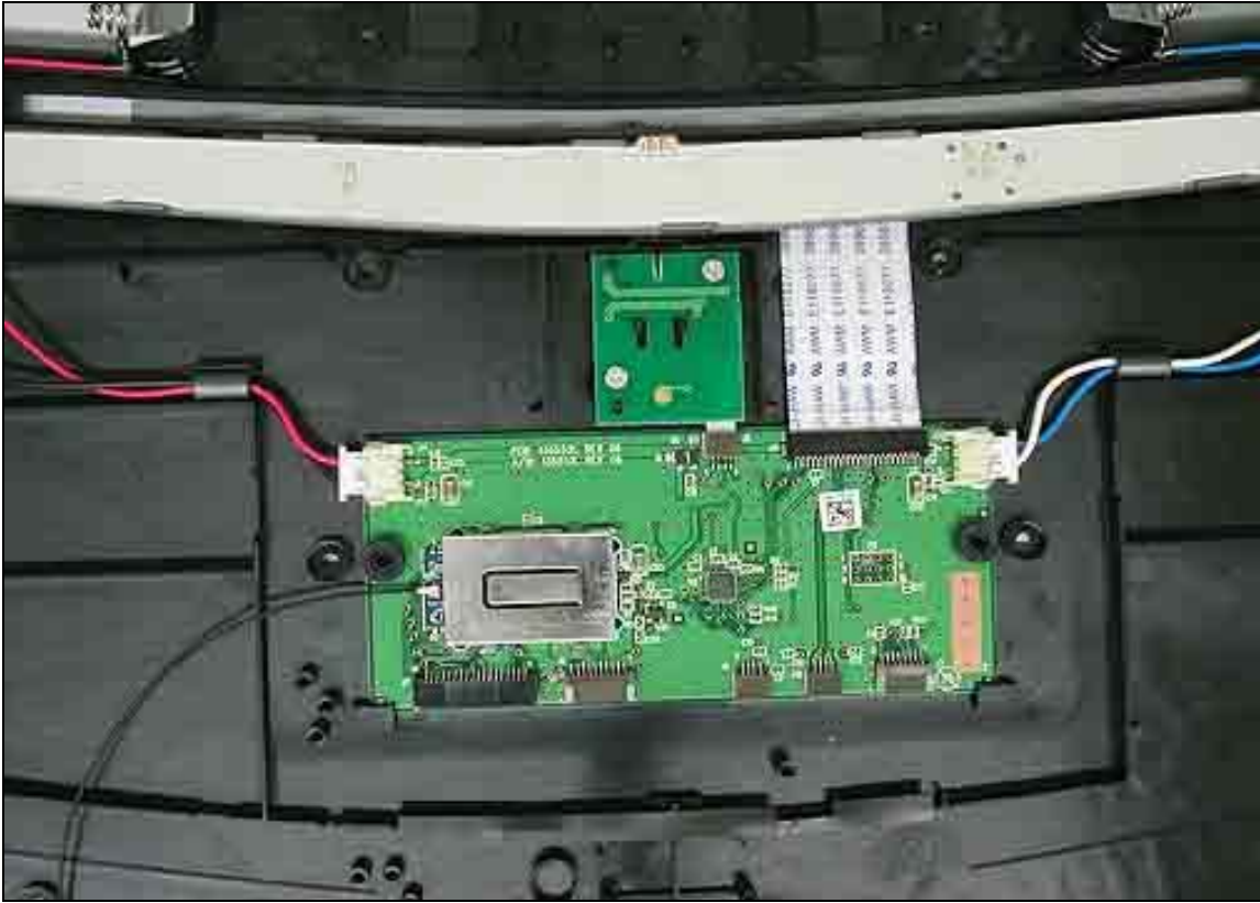
Main PCB Showing Ferrite Locations
