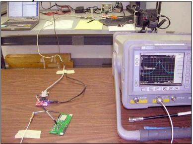
**Test Conditions:** The EUT is a bluetooth Keyboard. The keyboard is working and continuously sending an 'H' to a remotely located laptop computer. The keyboard is communicating with the laptop via a usb bluetooth adapter. The H key of the USB keyboard is continuously pressed and the H pattern is being displayed in Notepad. All data taken with this configuration. Bandwidth settings: 1MHz.
