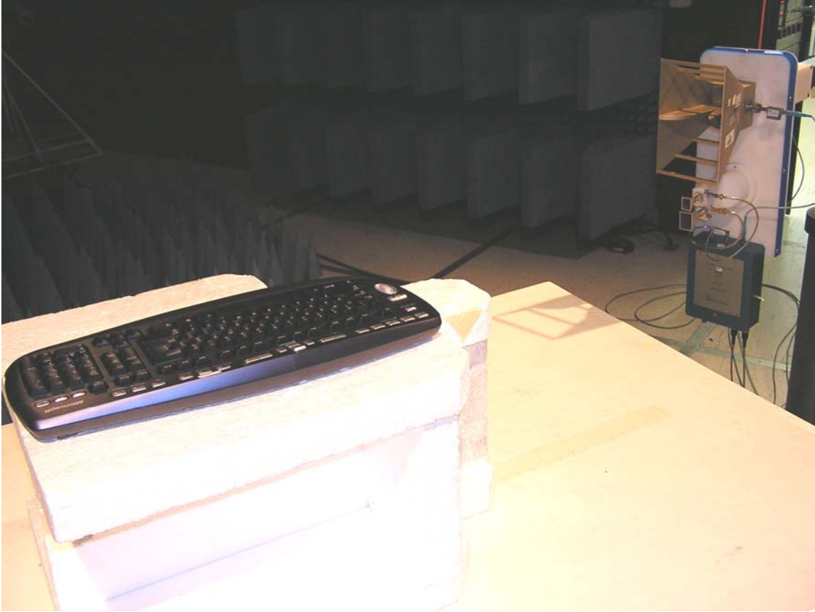
Test setup – Radiated Emissions
