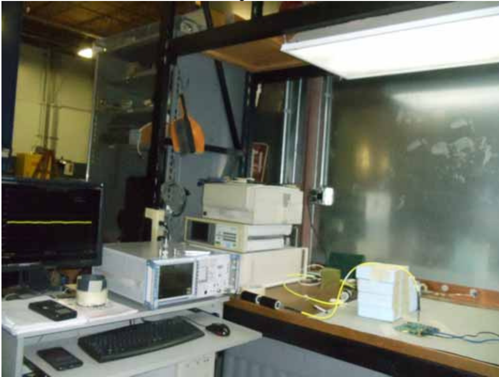
Test Setup for Antenna Conducted Emissions
