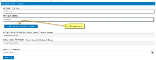
The WF-4000 will scan for available networks and display a list sorted by signal strength.
