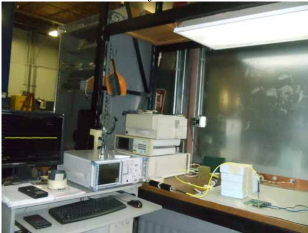
Test Setup for Antenna Conducted Emissions
