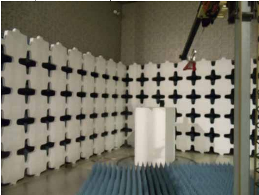
Test Setup for Radiated Emissions, above 1GHz to 18GHz – Vertical Polarization
