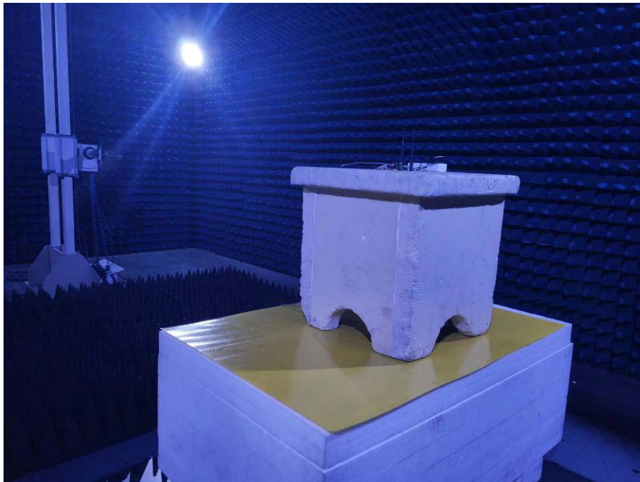
Photo of Radiated Emission Measurement Above 1GHz
