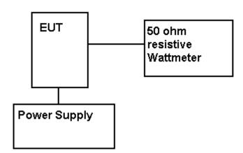
Part 2.1033 (C)(8) DC Input into the final amplifier
