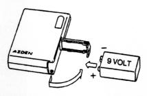
Open the battery compartment lid by sliding it down and raising the lid. Insert a 9 volt battery into the battery compartment with the correct polarity. Directions are on the inside left of the battery compartment.
