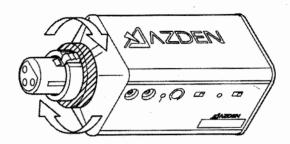
To plug the 51XT onto a microphone (low impedance with XRL connector) first make certain the locking-ring is turned fully up (rotate counterclockwise). Then plug the 51XT fully into the microphones XLR connector and tighten by rotating the ring fully down (clockwise).
