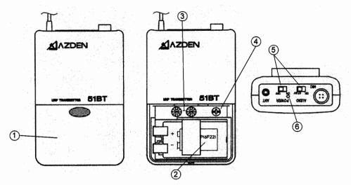
The **51BT** body-pack transmitter has 63 user selectable UHF frequencies and is ideal for lavaliere and headset microphones. The optional MP-1H instrument cable allows the 51BT to work with electric guitars and basses.
