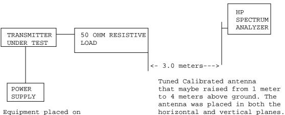
Equipment placed on rotating platform, 80 cm above ground.
