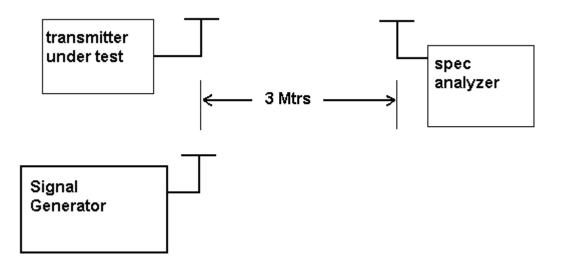
RF power is measured by the substitution method as outlined in TIA/EIA - 603. With a nominal battery voltage of 9.0V, and the transmitter properly adjusted, the RF output measures:
