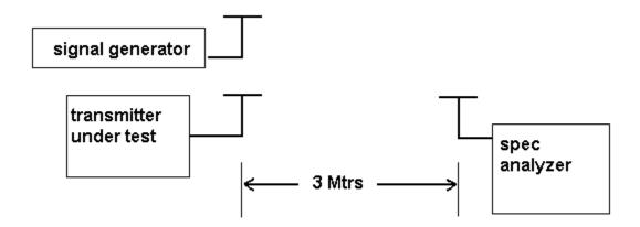
**METHOD OF MEASUREMENT:** The tabulated data shows the results of the radiated field strength emissions test. The spectrum was scanned from 30 MHz to at least the tenth harmonic of the fundamental. This test was conducted per ANSI/TIA 603-C:2004 using the substitution method. Measurements were made at the test site of Timco Engineering, Inc. located at 849 NW State Road 45, Newberry, FL 32669.
